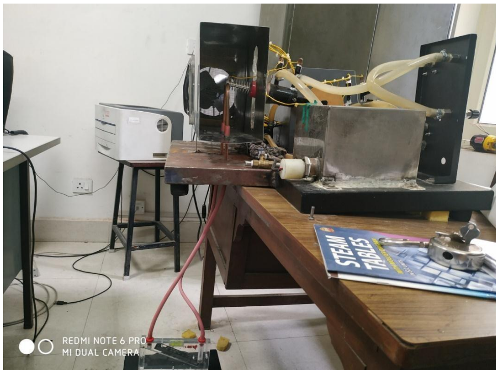
Figure 3.6. Pressure pipes through the base of the duct connected to single column inclined manometer
