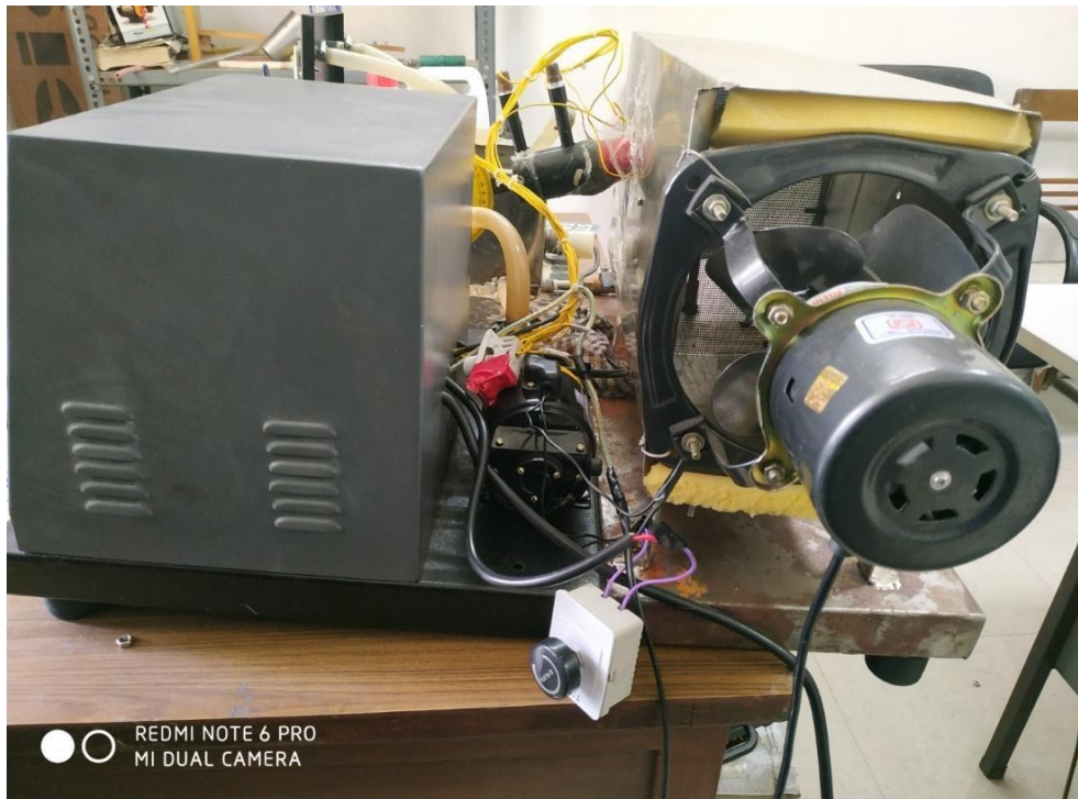
Figure 3.3. Fan mounted on a duct having a regulator
