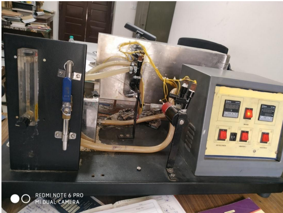
Figure 3.5. Front side Depicting Rotameter and By-pass valve
