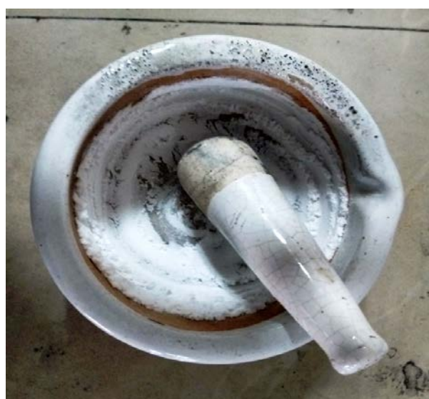
Figure 4.7: Mixing of salts at eutectic mixture
