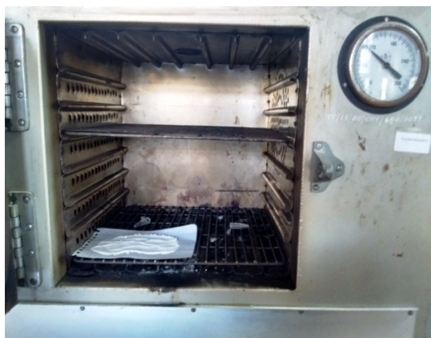
Figure 4.3: Heating of salt to evaporate moisture
