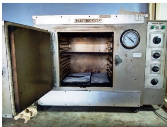
Figure 4.10: Heating of salt to evaporate moisture
