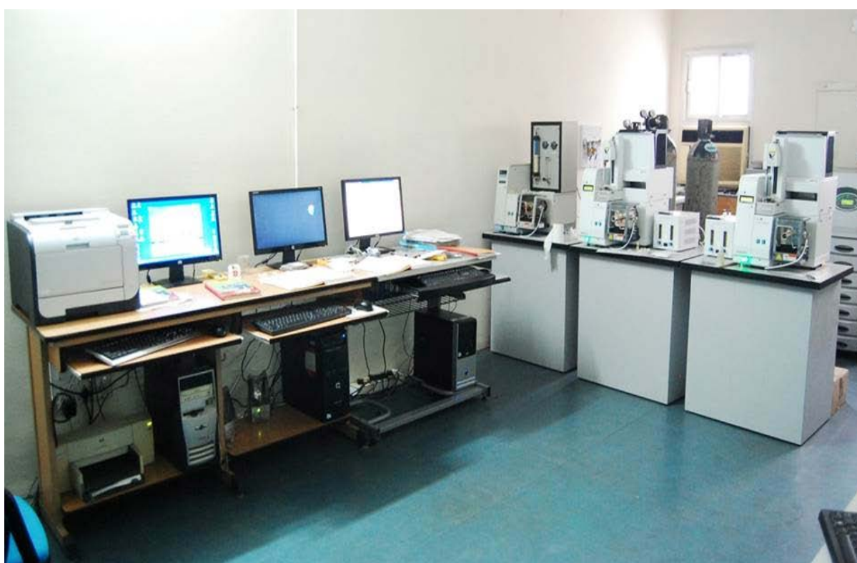
Figure 4.12: TG/DTA (EXSTAR SII 6300) facility at IIT Roorkee
