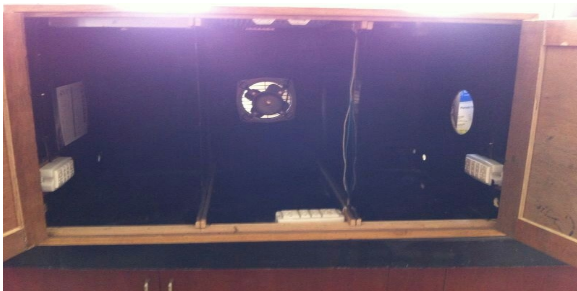
Fig 3.1 Lab scale UV LED reactor showing the partitions(Front view)
