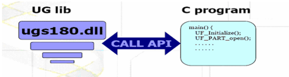
Fig: 2.8. Interfacing of C with UG library using API [39]
