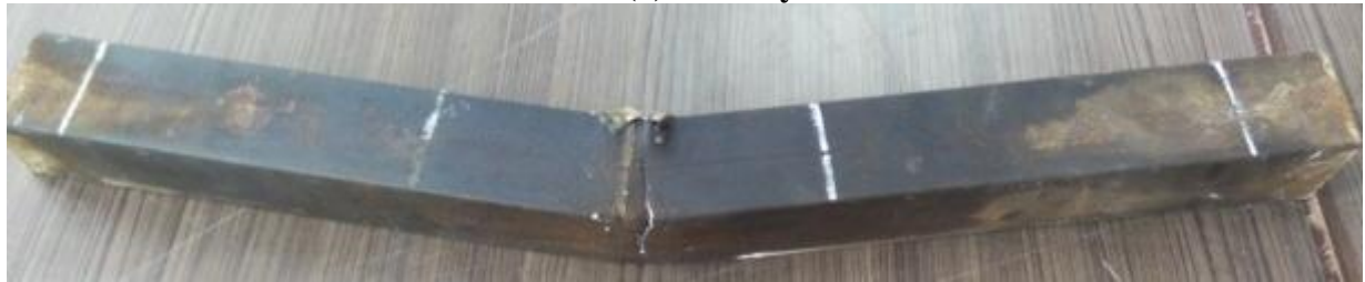
(b) 8 Days corrosion
