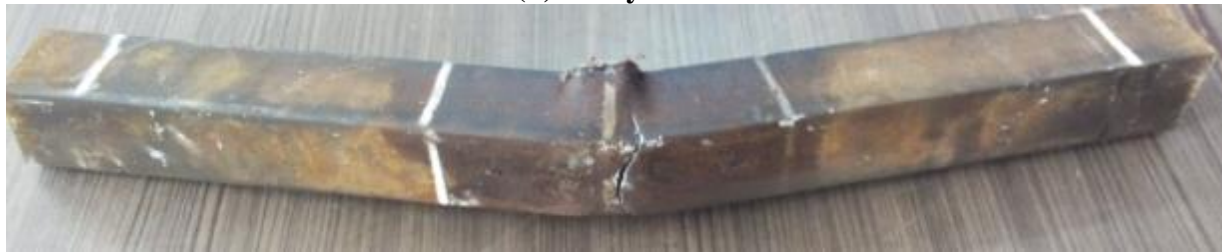
(c) 6 Days corrosion
