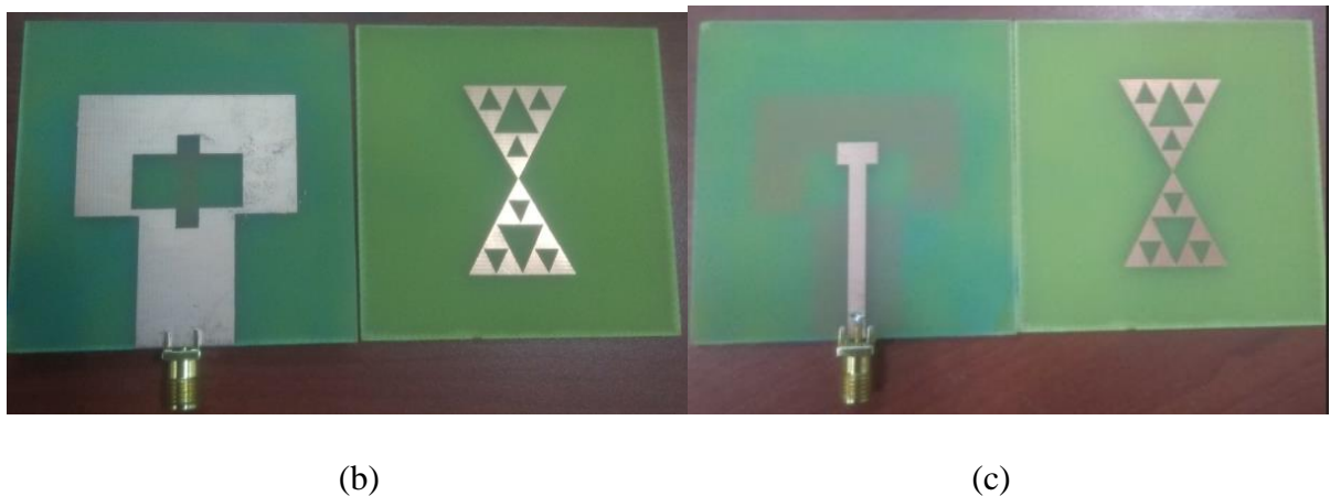
Figure 5.2 Photograph of fabricated antenna (b) partial ground and top perspective of fabricated antenna, (c) strip line and the active patch of the fabricated antenna
