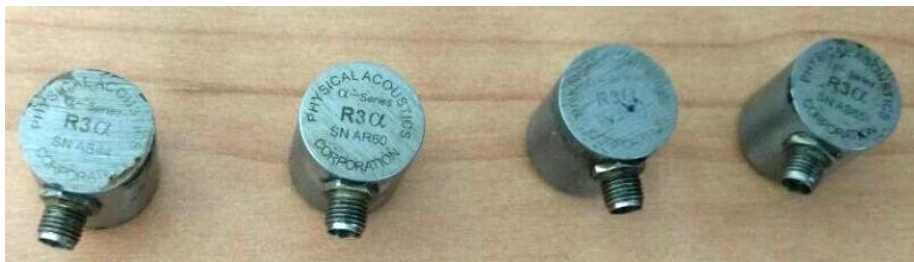
Fig.3.15: R3 \alpha Sensors for acquisition of data
