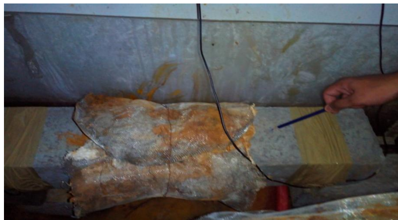
Fig.3.19: Pencil break test during study
