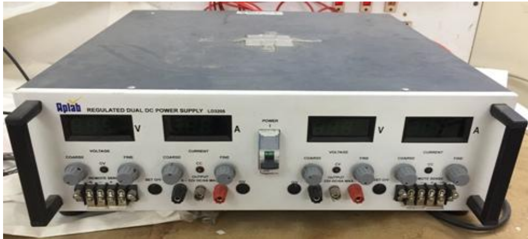
Fig. 3.7: Power supply (Aplab, 64V, 1A Current)
