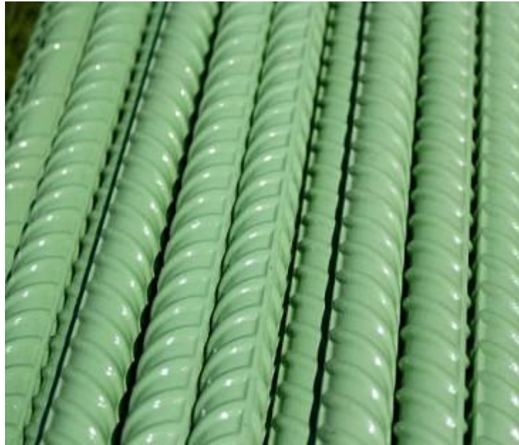
Fig.1.2: Steel bar coated with epoxy [1]
