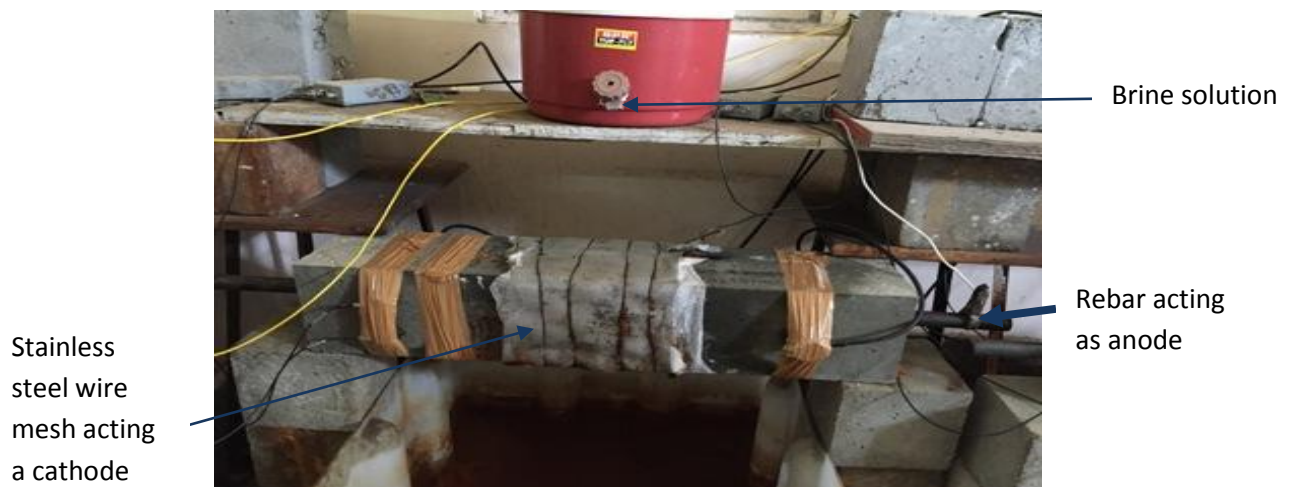
Fig.3.6: Beam showing arrangement for induced corrosion
