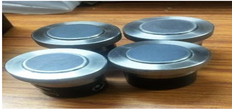
Fig.3.11: Transducers used (Karl Deutsch, 0.1 MHz and 1MHz)
