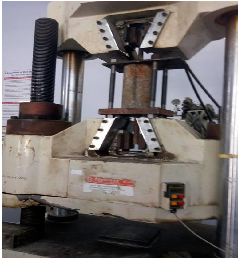
Fig. 6.19: Pull-out test set-up
