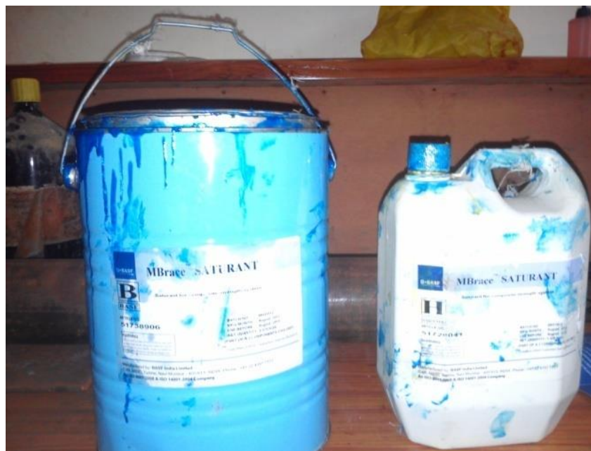
Fig. 5.7: MC Brace Adhesive used for bonding FRP with concrete
