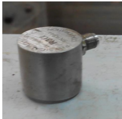
Fig.5.18: R3a Sensors for AE Acquisition used in the study.
