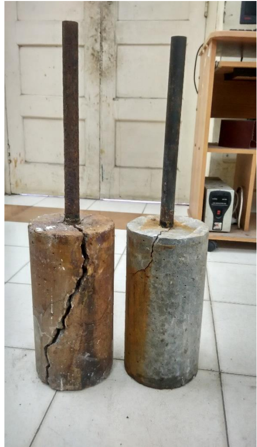
Fig 5.3 Cylindrical Specimen after corrosion
