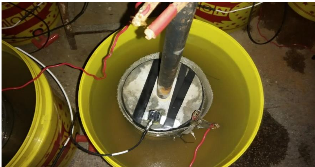
Fig.5.22: Actual sensors mounted on the cylinder
