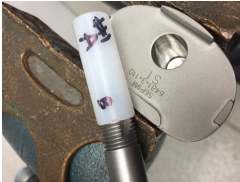
Figure 7.21: Removal tool engaged with poly sleeve
