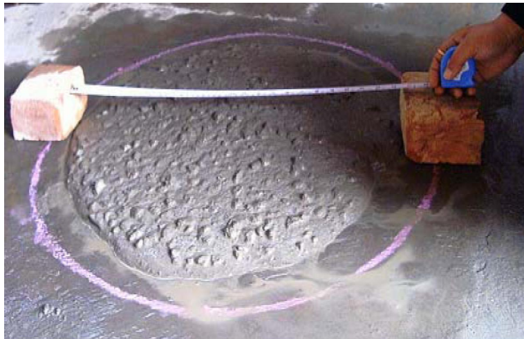
Figure 2.2 Measuring of Diameter
