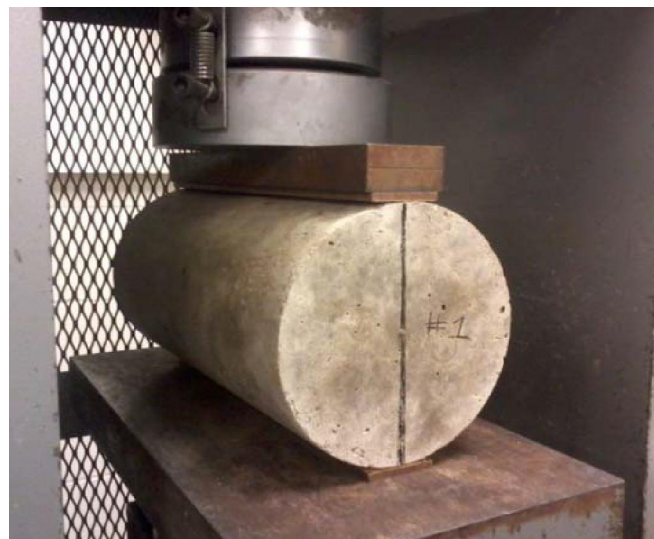
Figure 2.11 Splitting Tensile Test
