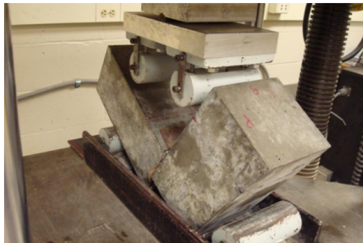
Figure 2.10 Post Failure Specimen
