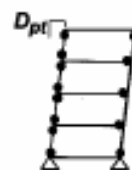
(b) Total Mechanism with Weak Columns
