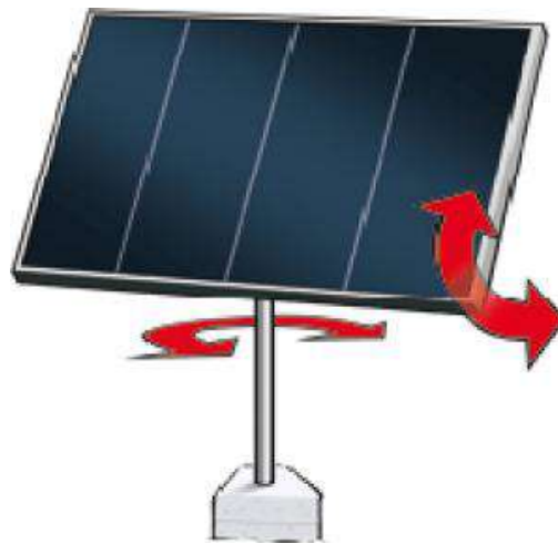
Figure 1.6 Double axis solar tracker [Cheema, S S 2012]
