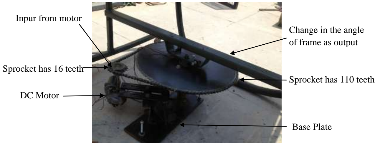
Figure 4.9 Automatic Horizontal Tracking Mechanism
