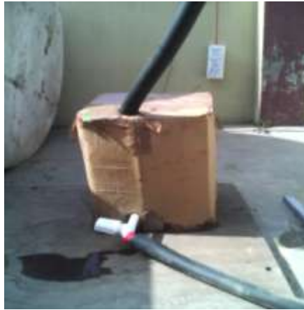
Figure 4.4 Storage Tank insulated with Glass wool and packed in Box
