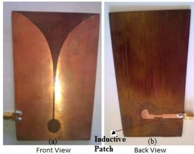
Fig.7.6 Fabricated design of Vivaldi Antenna (a) front view. (b) Back view showing feeder with Compensation (Inductive Patch on feedline).
