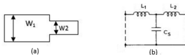
Fig.7.1 (a) Shows the layout of reactive patch in the feed line. (b) Represents the equivalent circuit diagram of reactive patch.
