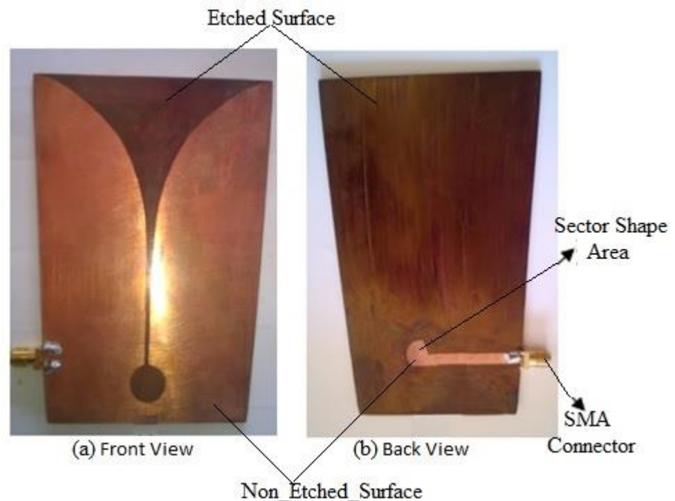
Fig.6.1. The diagram shows the front and back view of Vivaldi antenna fabricated on PCB.
