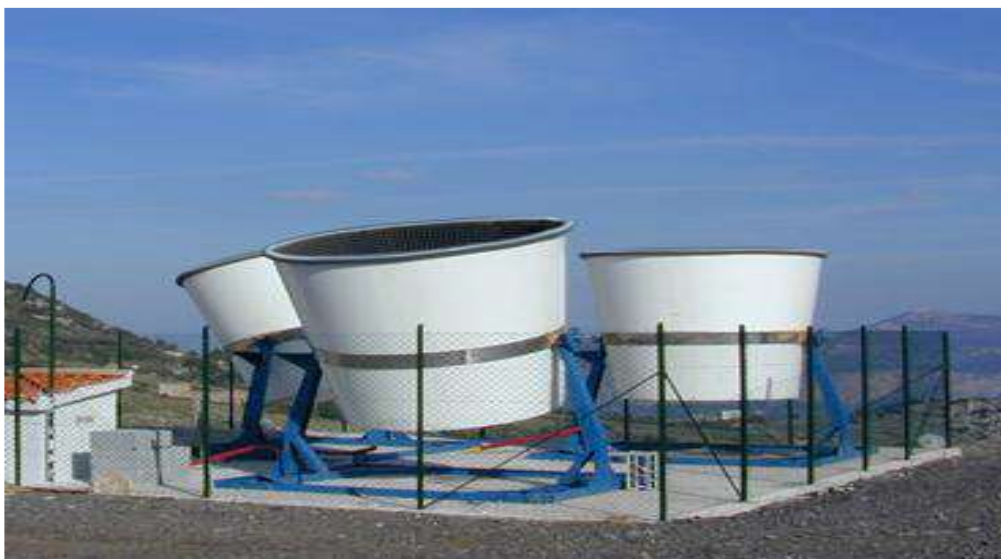
Figure 2.3. Three axis Doppler SODAR
