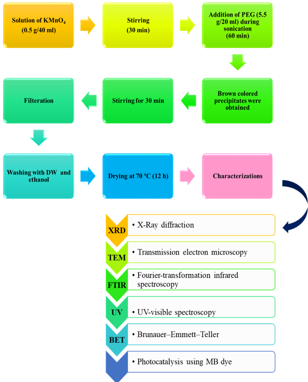
Figure 3.1: Flow chart for the synthesis of MnO 2 nanopowder.
