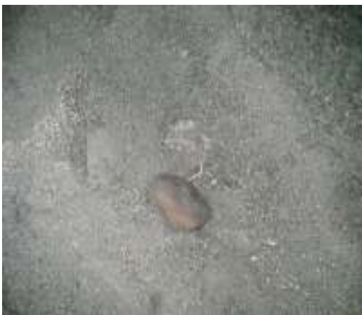
Figure 5.8 Hard agglomerate when (rice husk-rice straw is used) at JPP
