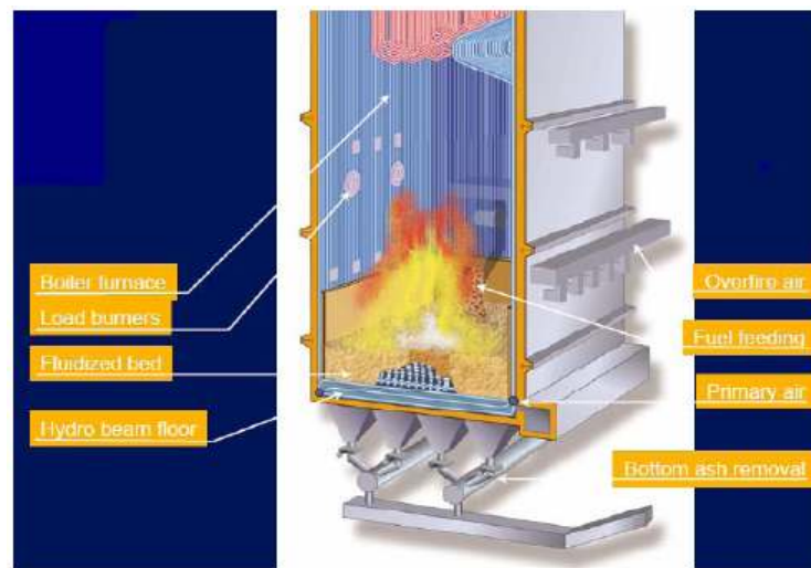
Figure 1.6: A view of atmospheric fluidized bed combustor [184]
