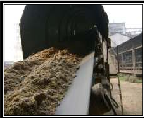
Figure 3.1 Fuel input to combustor through conveyor belt at JPP
