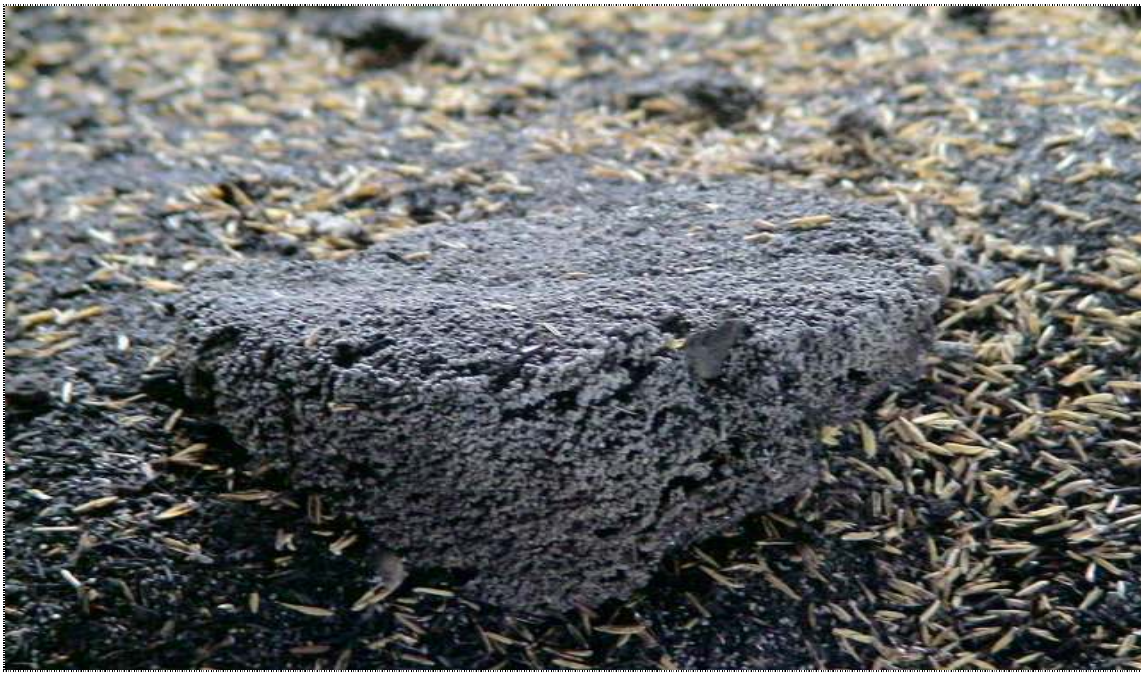
Figure 5.4 Ash agglomerate sample at JPP
