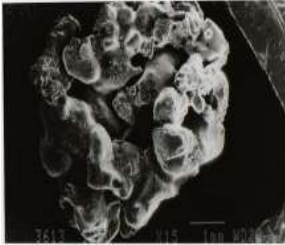
Figure 5.12 SEM of agglomerate sample Figure 5.13 SEM of two coalesced sand particles
