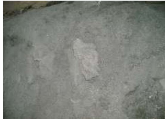
Figure 5.7 Agglomerate at bottom of furnace of JPP
