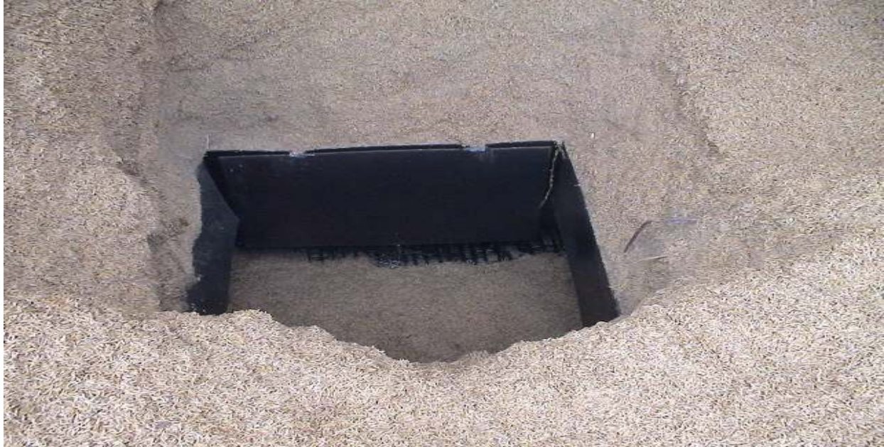
Figure 3.12 Feeding of rice husk through pile on to the conveyor belt at CPPDK
