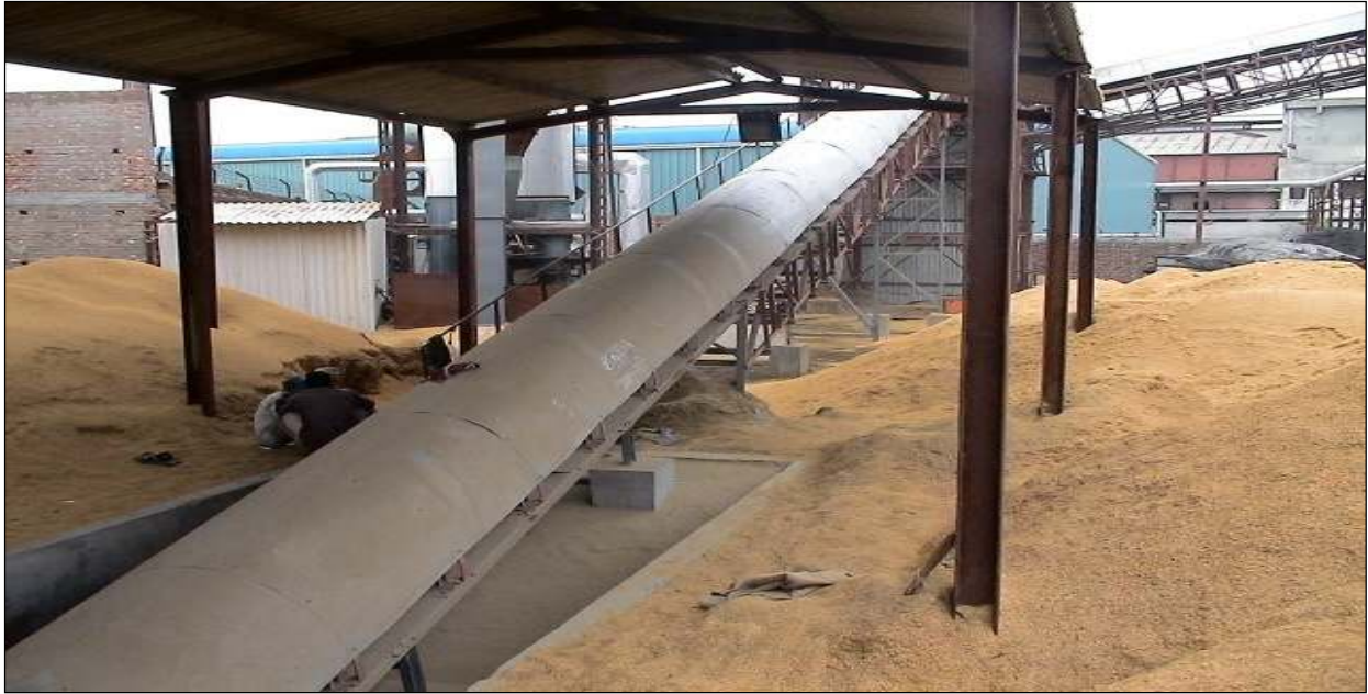
Figure 3.10 Feeding of rice husk to the atmospheric fluidized bed combustor through the conveyor belt at CPPDK
