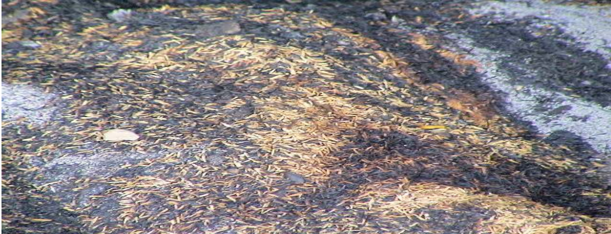
Figure 3.8 Unburnt rice husk along with bed ash
