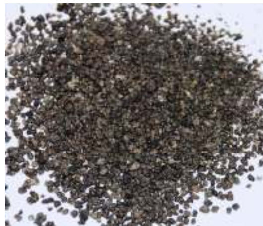
Figure 5.9 Cleaned sand for reusing at JPP
