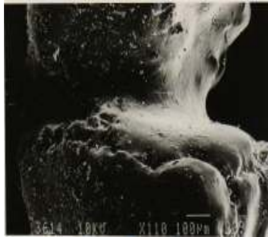
Figure 5.12 SEM of agglomerate sample Figure 5.13 SEM of two coalesced sand particles
