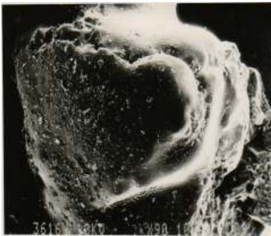
Figure 5.14 Sand particles showing rice husk ash-derived coating
