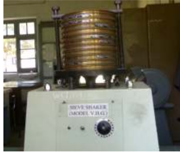
Figure A.3.2 Sieve shaker (Model-VGH, M/s. Versatile Equipments Pvt. Limited, Kohlapur, India)
