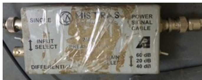
Fig. 5.15:Preamplifier used in the study (Mistras)
