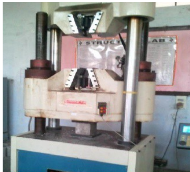
Fig.5.3: Sample in Universal Testing Machine
