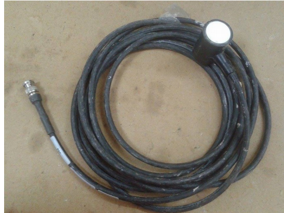
Fig. 5.14: R3 \alpha sensors used in the study
