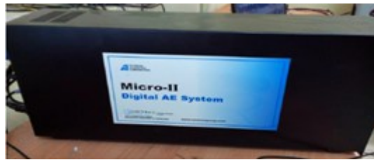
Fig. 5.16: AE data acquisition system (Micro II , Digital AE system)
