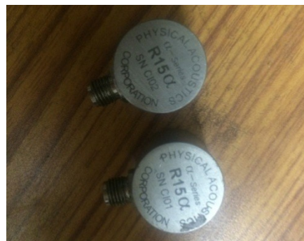
Fig. 5.13: R15 \alpha sensors used in the study
