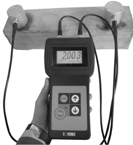
Fig.1.5: Ultrasonic pulse velocity test apparatus ( http://www.controls-group.com )
