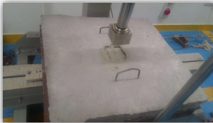
Fig. 6.4: Punching shear occurring on top surface of the slab
