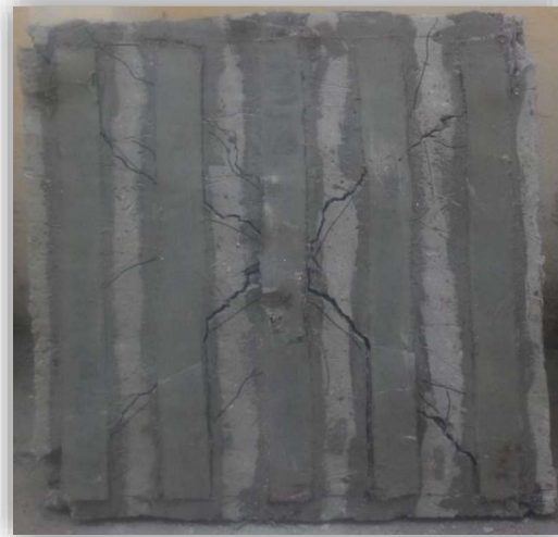
Fig. 6.10: Crack Pattern in FS 15 GFRP UD
