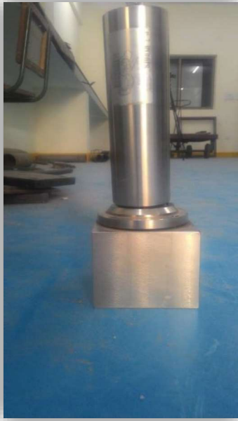
Fig. 6.2: Punching Failure Equipment
