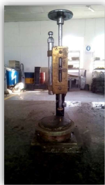
Fig. 3.2: Vicat Apparatus for testing Initial setting time
