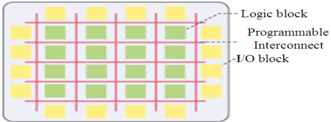
Figure 4.2: Internal Structure of an FPGA
