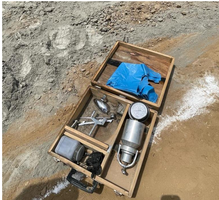
Figure 4.7: Moisture Meter for field moisture content.
