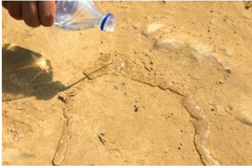
Figure 4.13: Waterproofing effect on compacted chemically treated sub-base
