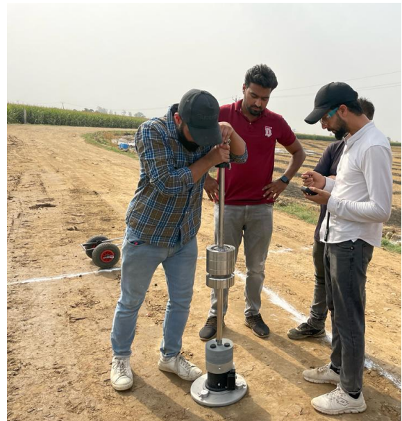
Figure 4.15: Marking of points for LWD test.
