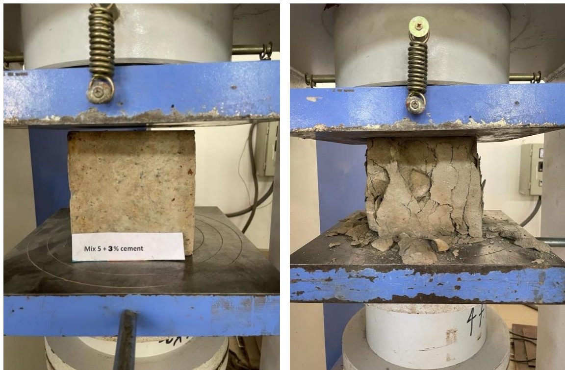
Figure 3.22: (i) Sample before loading (ii) Sample after loading
