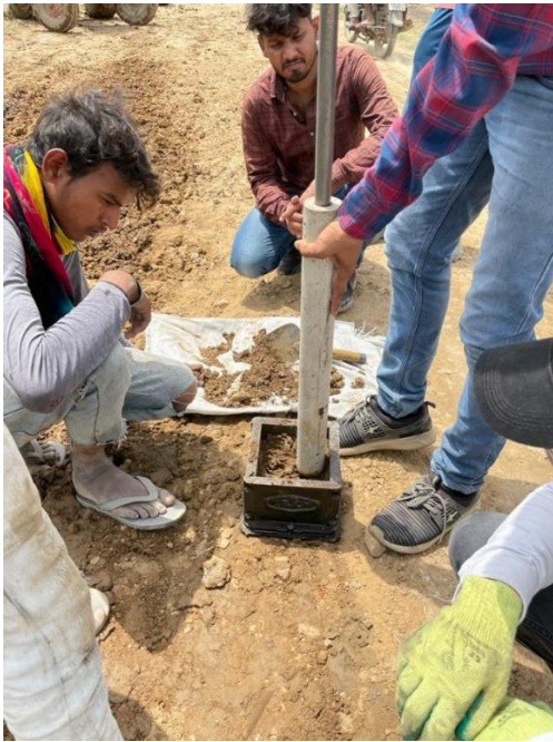
Figure 4.10: Collection of samples for UCS from field using (i) Heavy Hammer (ii) DLC Hammer
