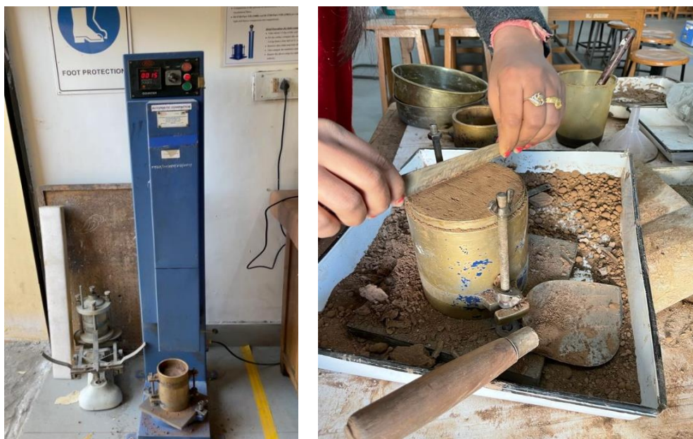
Figure 3.14: OMC/MDD of soil using automatic compactor.
