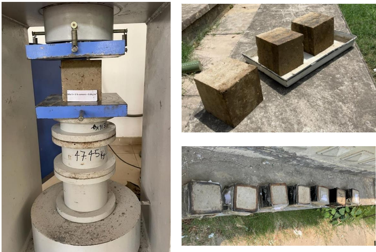
Figure 3.17: ACTM machine, Samples for UCS testing.
