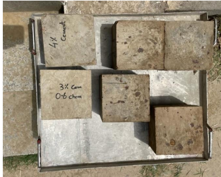
Figure 4.12: Samples for 7-day UCS testing
