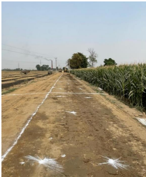
Figure 4.15: Marking of points for LWD test.
