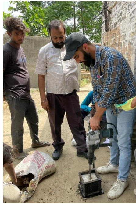
Figure 4.10: Collection of samples for UCS from field using (i) Heavy Hammer (ii) DLC Hammer
