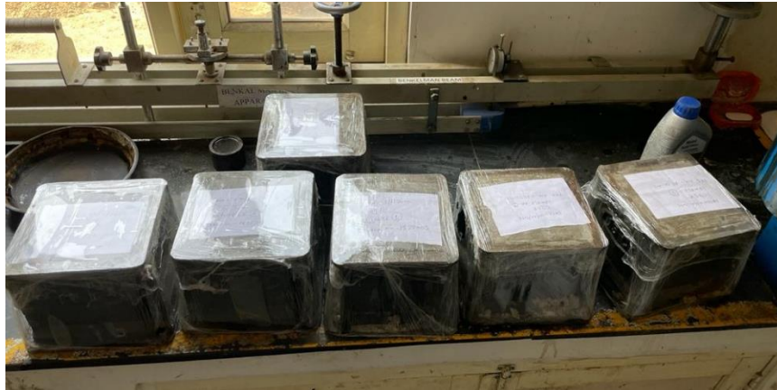
Figure 3.19: Moulds wrapped with plastic sheets
