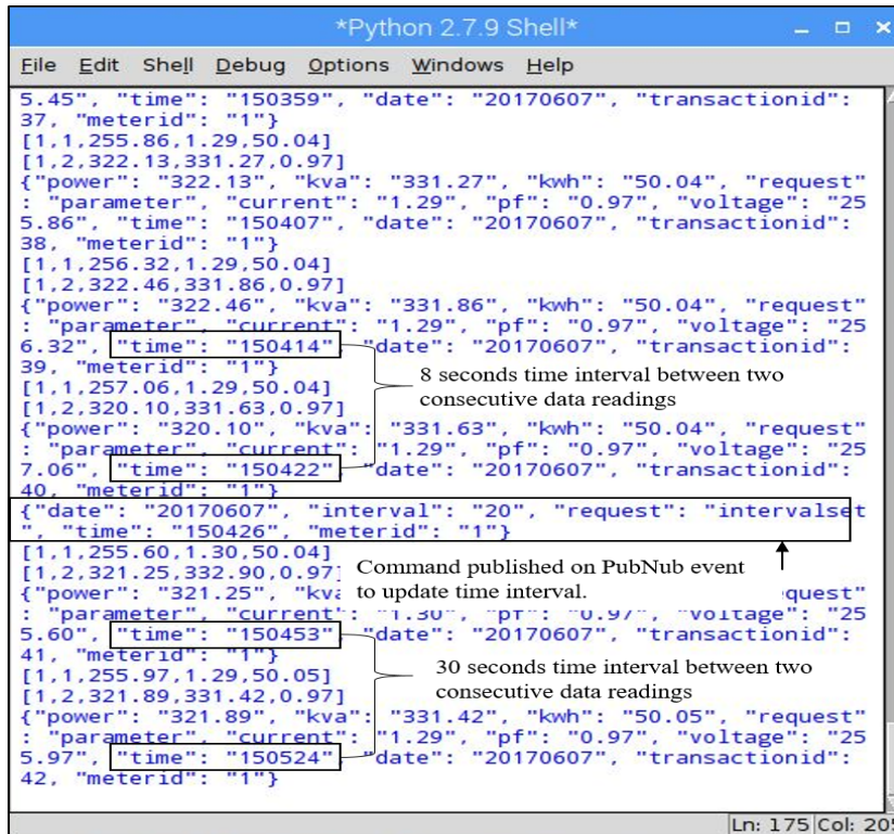
Fig. 5.6: Set Time Interval of consecutive data readings from Remote server using GUI
