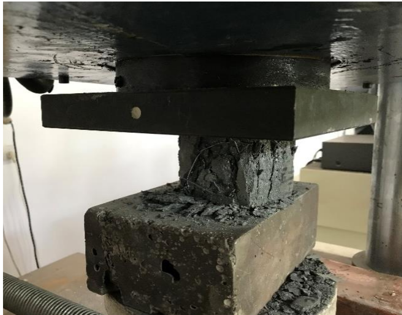
Fig. 3.17 – Failure Pattern of 28 Days Cured HPHFRC-2 Sample (Phase- III)
