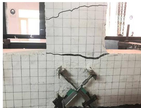
Fig. 5.12 - Crack Pattern of Control Slight Damage (C-SD) Specimen II
