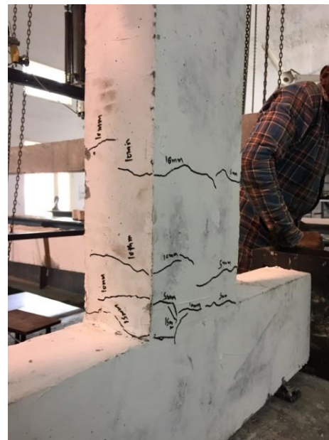
Fig. 6.11 - Side View of the Crack Pattern of Control Moderate Damage (CMD) Specimen I
