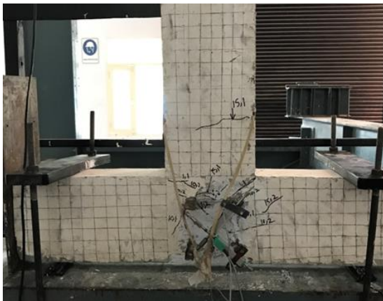
Fig. 5.8 - Crack Pattern of Control Moderate Damage (C-MD) Specimen I
