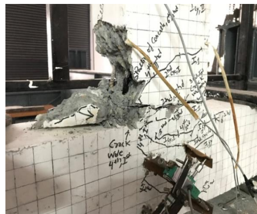
Fig. 6.3 - Concrete Spalling at the Ultimate Lateral Displacement of Control Complete Damage (CCD) Specimen I
