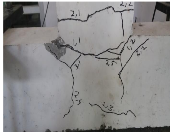
Fig. 5.9 - Crack Pattern of Control Moderate Damage (C-MD) Specimen II
