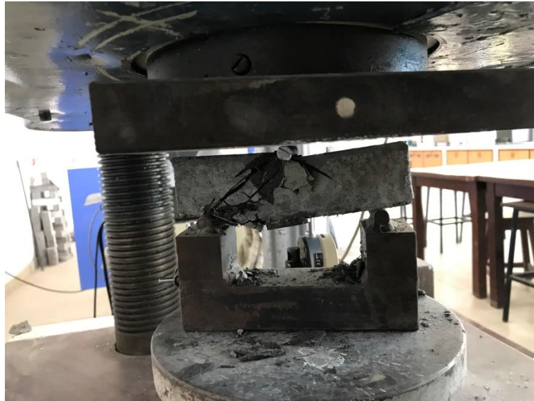
Fig. 3.35 - Ultimate Failure of HPHFRC-SC Specimen during Flexural Testing
