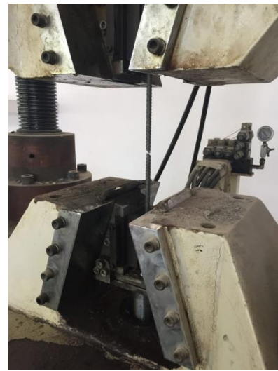
Fig. 4.4 - Ultimate Fracture of Reinforcement
