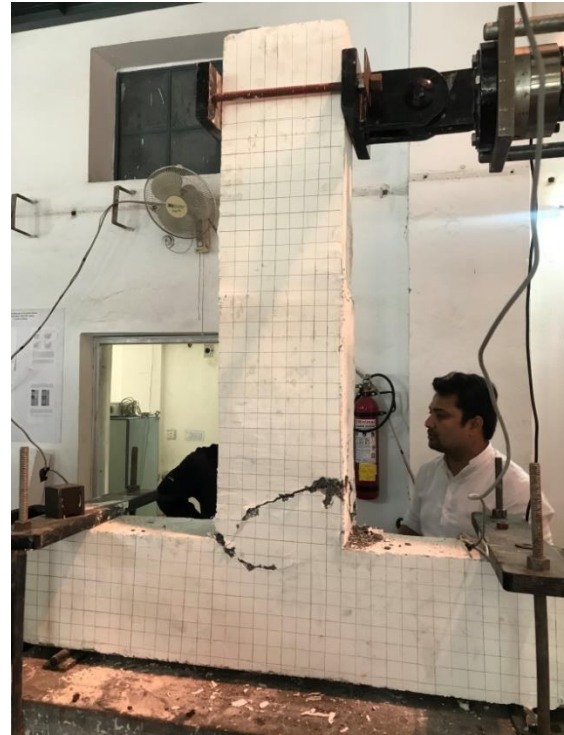
Fig. 6.34 - Crack Extended on the Back Side of the Wire Mesh Confined HP-HFRC Retrofitted Control Complete Damage (WC-RCD) Specimen I
