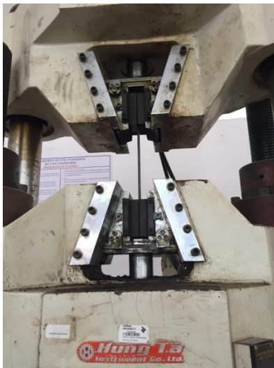
Fig. 4.3 - Testing Arrangement of Reinforcement
