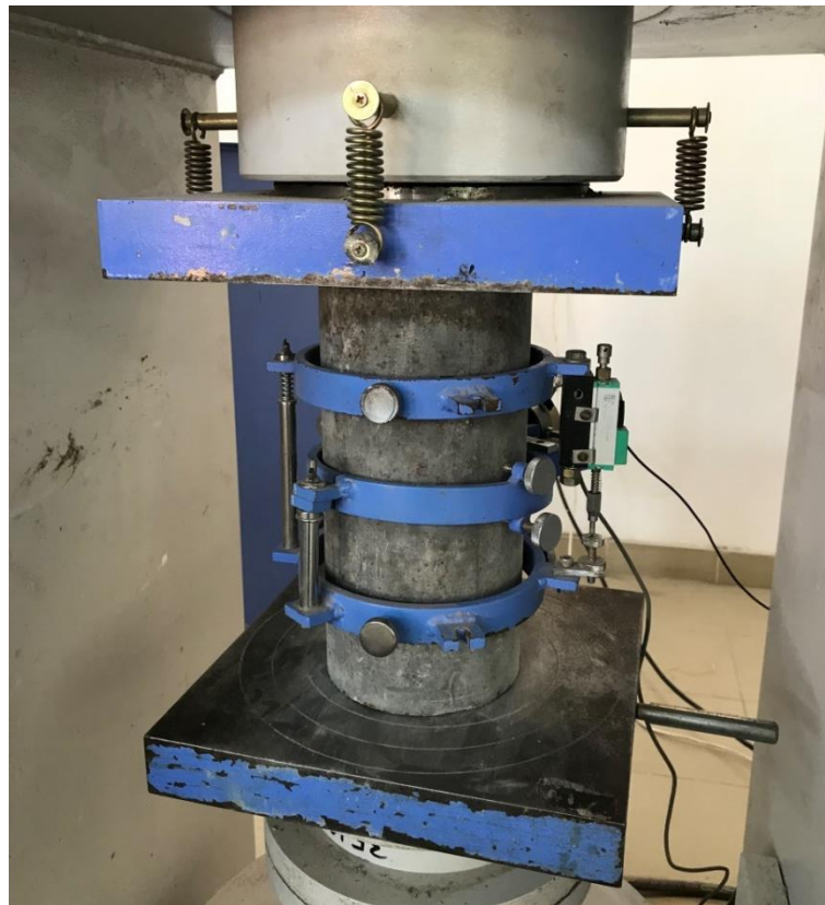
Fig. 3.10 - Test Setup to Evaluate the Stress Strain Behaviour of HPC/HP-HFRC
