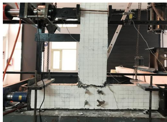
Fig. 5.35 - Failure Pattern of R-SED at Ultimate Lateral Displacement (Specimen 2)
