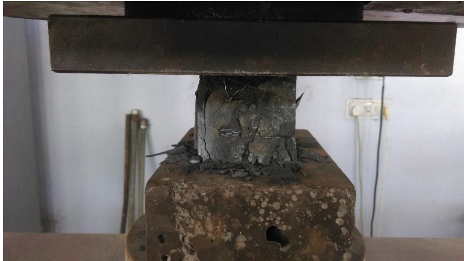
Fig. 3.9 – Test Setup used to Test the Compressive Strength of HPC/HP-HFRC
