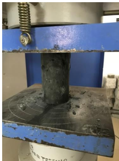
Fig. 3.29 - Compressive Strength Test Setup
