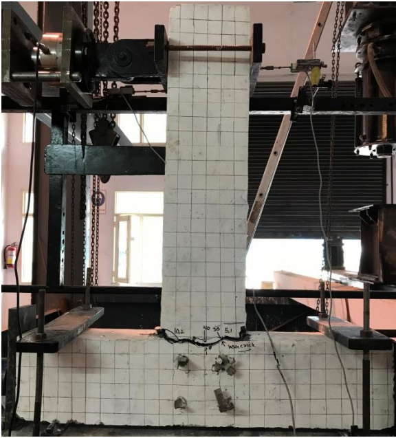
Fig. 6.37 - Crack Pattern of Wire Mesh Confined HP-HFRC Retrofitted Severe Damage (WC-RSED) Specimen I
