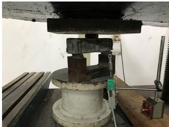
Fig. 3.11 – Three Point Bending Test Setup Arrangement
