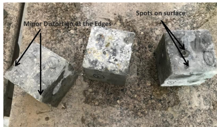
Fig. 3.39 - Visual Inspection of HPHFRC-SC Specimen after 180 Days Curing in Sodium Sulphate Solution
