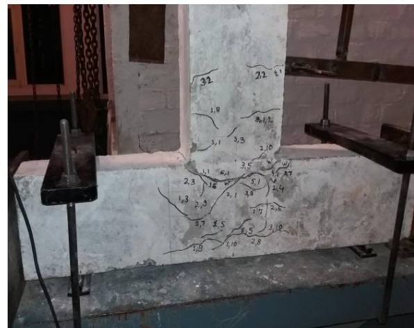
Fig. 5.6 - Crack Pattern of Control Severe Damage (C-SED) Specimen II
