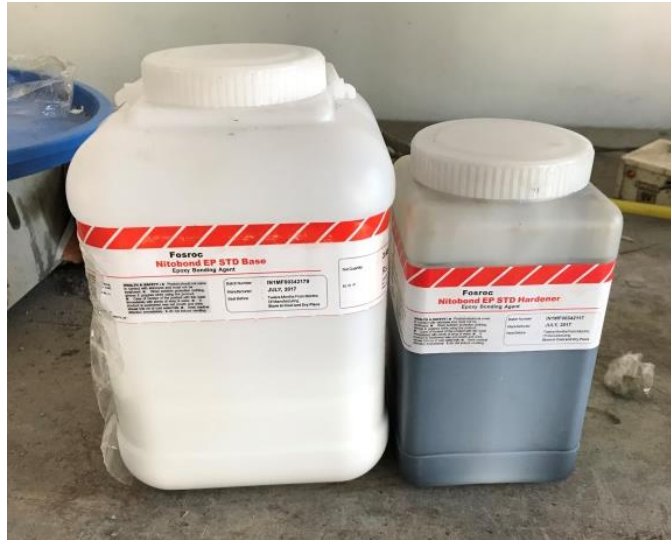
Fig. 4.5 - Nitobond EP STD used for Offering the Efficient Bond between Old and New Concrete
