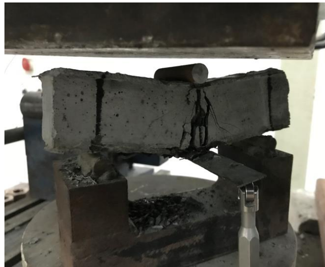
Fig. 3.34 - Large Crack Width of HPHFRC-NC Specimen Obtained during Flexural Testing
