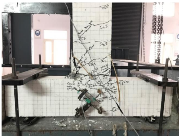
Fig. 6.2 - Crack Pattern of Control Complete Damage (CCD) Specimen I
