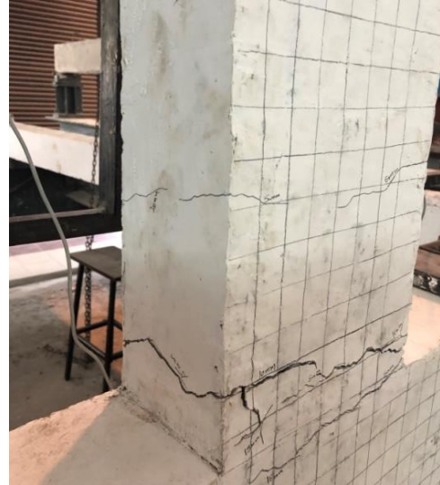
Fig. 6.13 - Side View of the Crack Pattern of Control Moderate Damage (CMD) Specimen II
