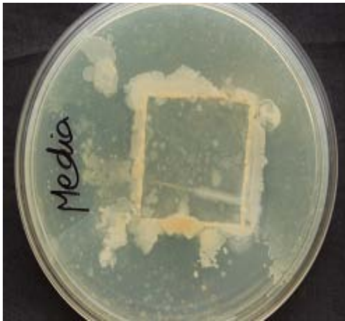
Figure 4.2 Photograph of the petriplate showing polymer kept in centre of NA plate
