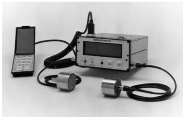
Fig 3.6 Pulse velocity instrument. (Courtesy of James Instruments, Inc.)
