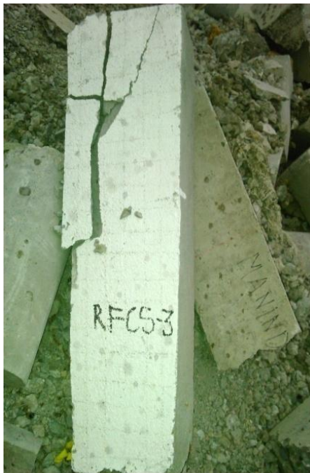
Fig. 4.4 Crack pattern after failure (RFCS)
