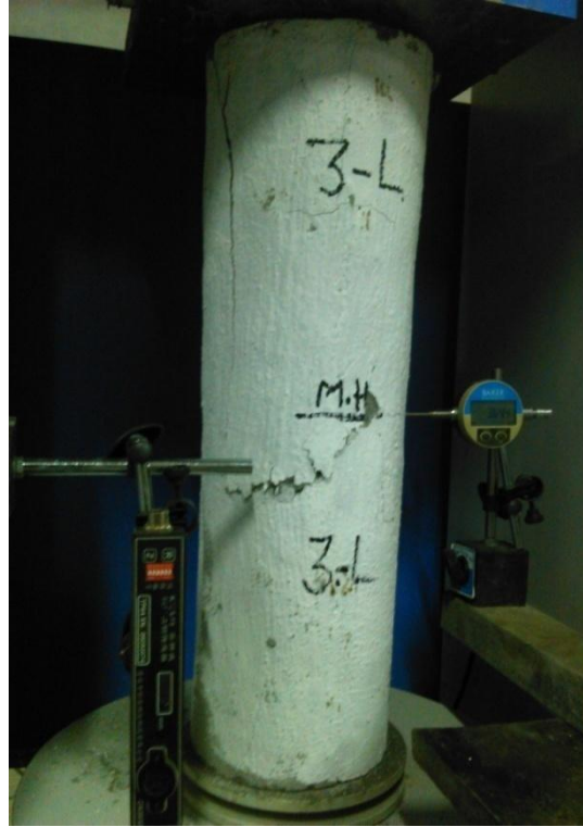
Fig. 4.19 Failure of Circular Column Confined with Three Layers of GI Wire Mesh (CC 3)
