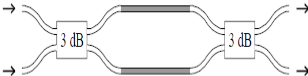
Fig 1.2 Mach-Zehnder interferometer based switch
