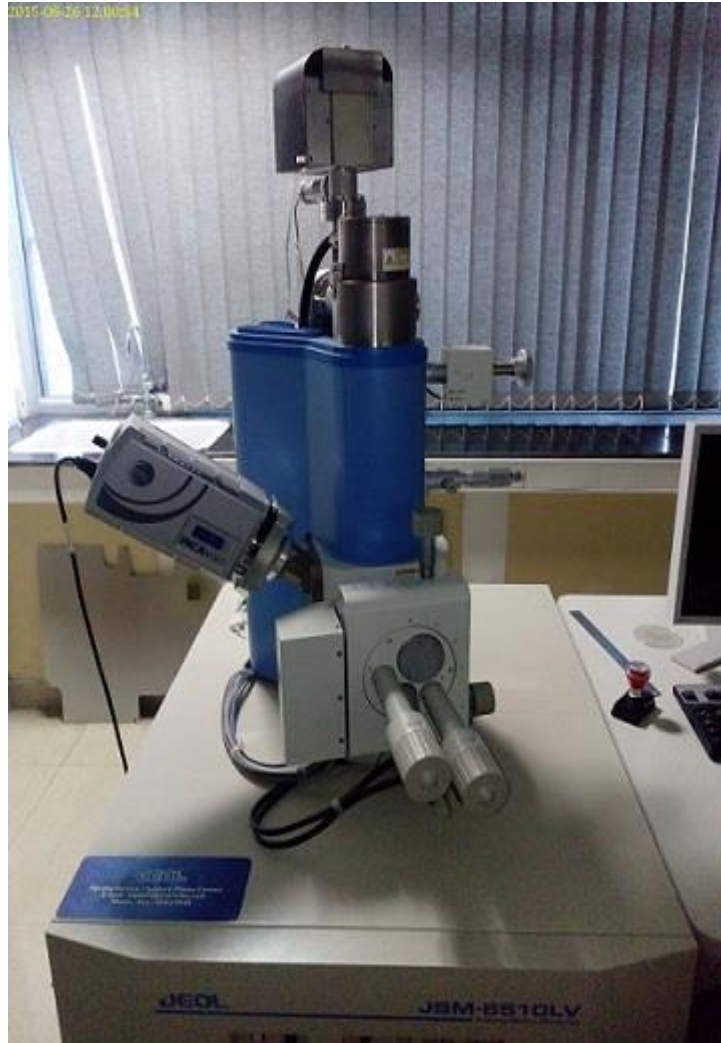
Figure 3.8: Scanning Electron Microscope (Courtesy: SAI Lab, TIET, Patiala)
