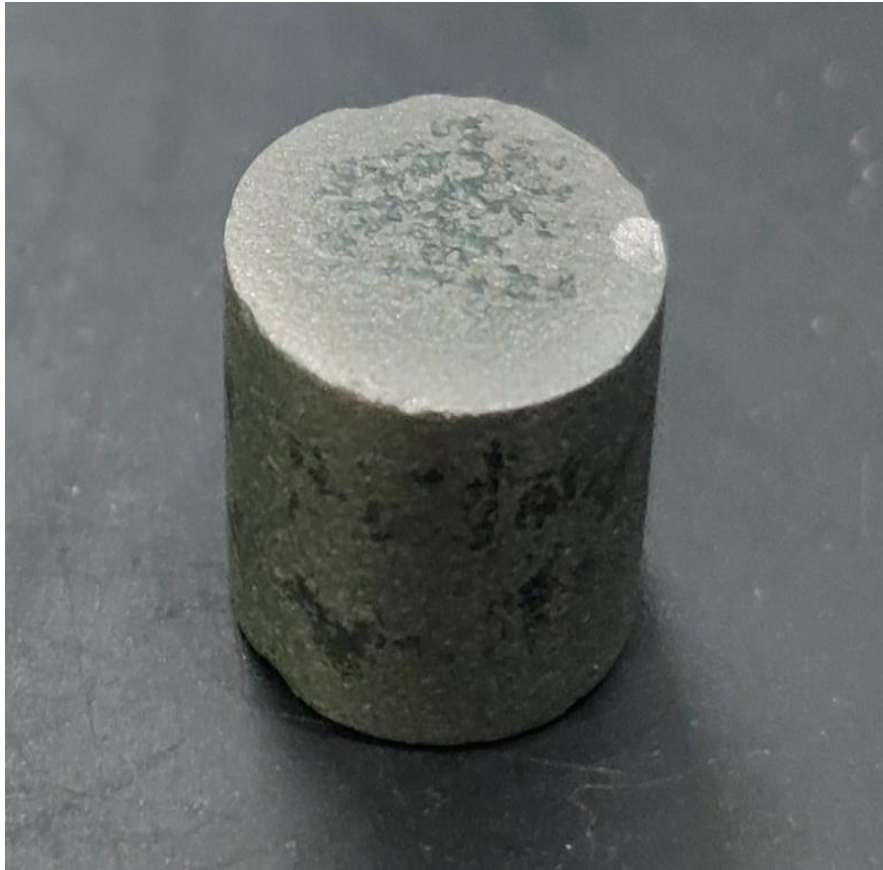
Figure 3.2: Ti6Al4V-Graphene composite prepared using SPS process
