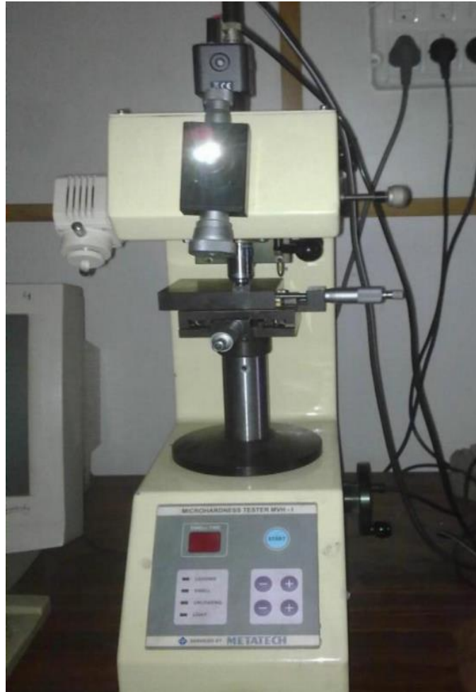
Figure 3.6: Micro hardness tester Model: MVH2 (Courtesy: Advanced Measurement Lab, TIET, Patiala)
