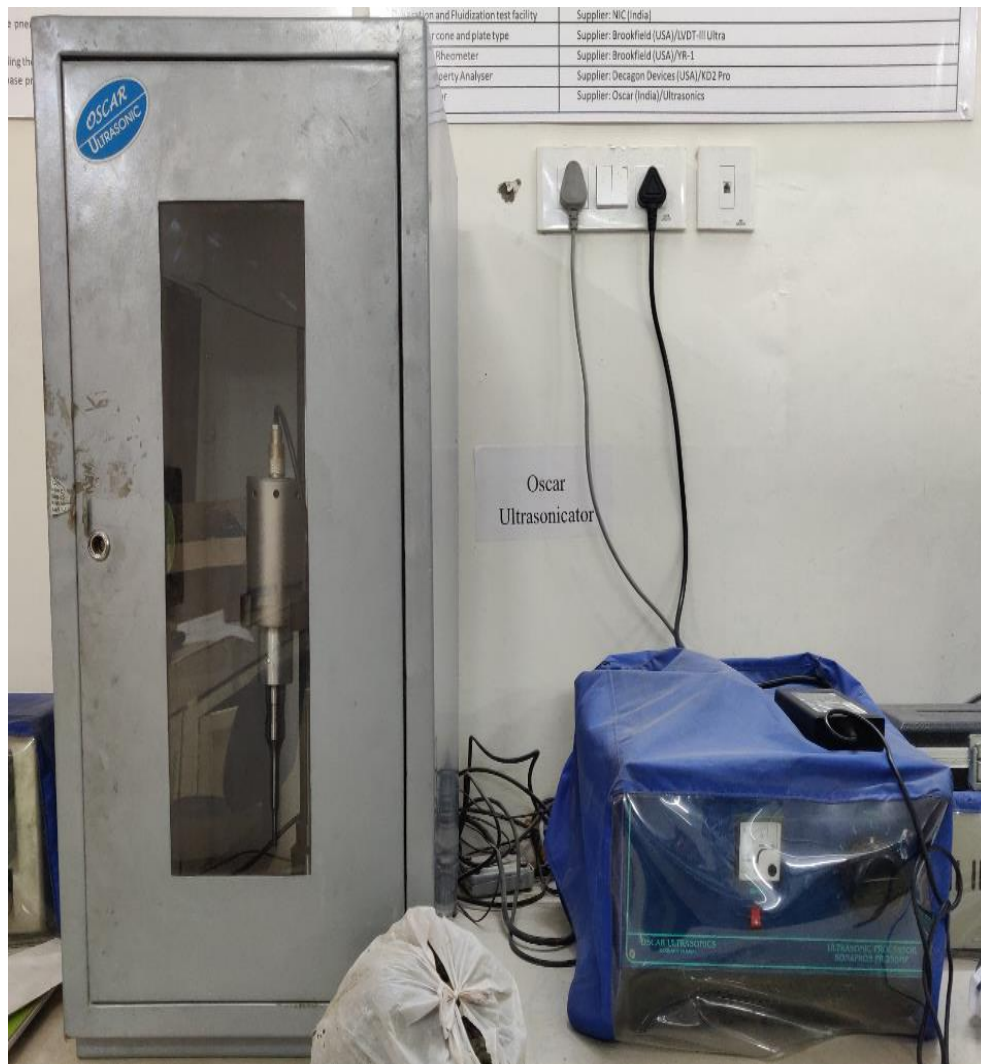
Figure 3.3: Oscar ultrasonicator (Courtesy: TIET, Patiala)
