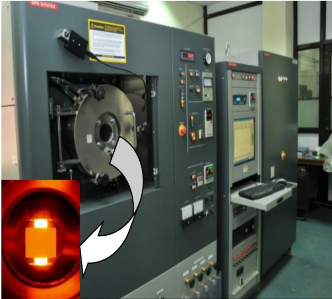
Figure 3.4: Spark Plasma Sintering Setup (Courtesy: CSIR-National Physical Laboratory, Delhi)
