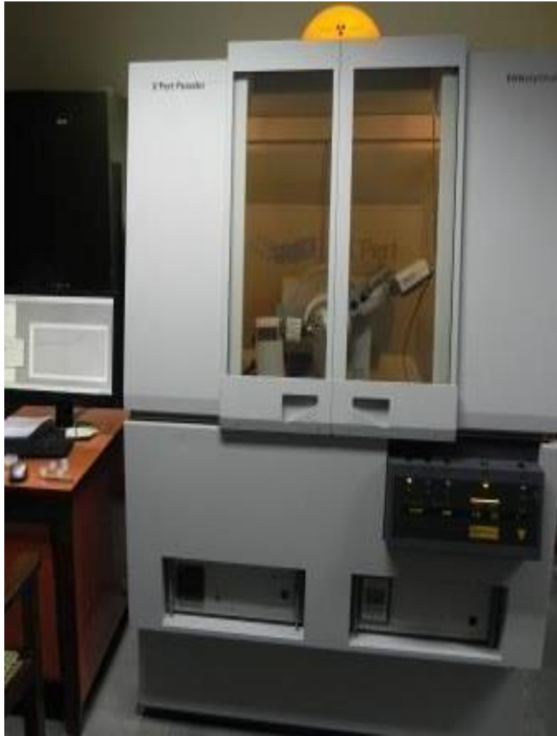
Figure 3.5: X-RAY Diffraction (Courtesy: SAI Lab, TIET, Patiala)
