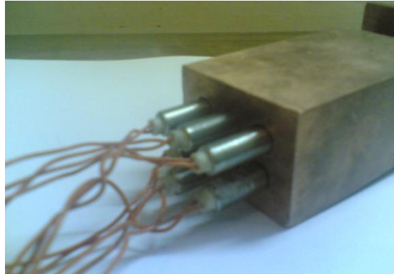
Fig. 3.24: Cartridge heaters fitted in copper block
