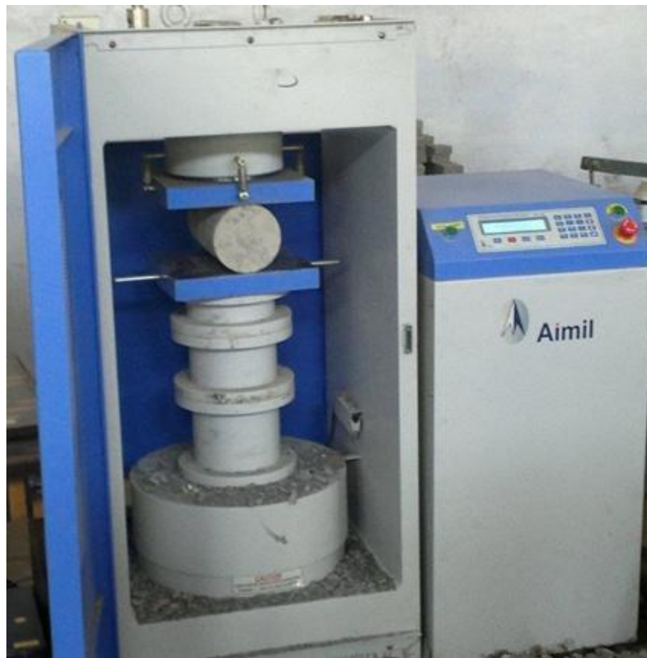
Fig. 3.5 Testing of cylindrical specimen
