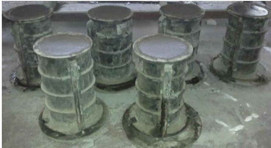
Fig. 3.6 Casting of cylindrical specimens
