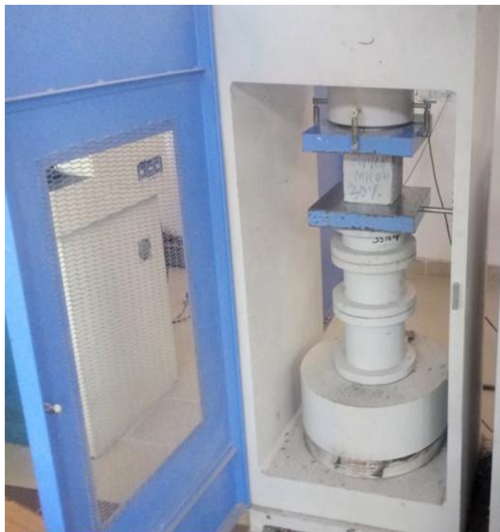
Fig. 3.4 Compressive strength testing of cube
