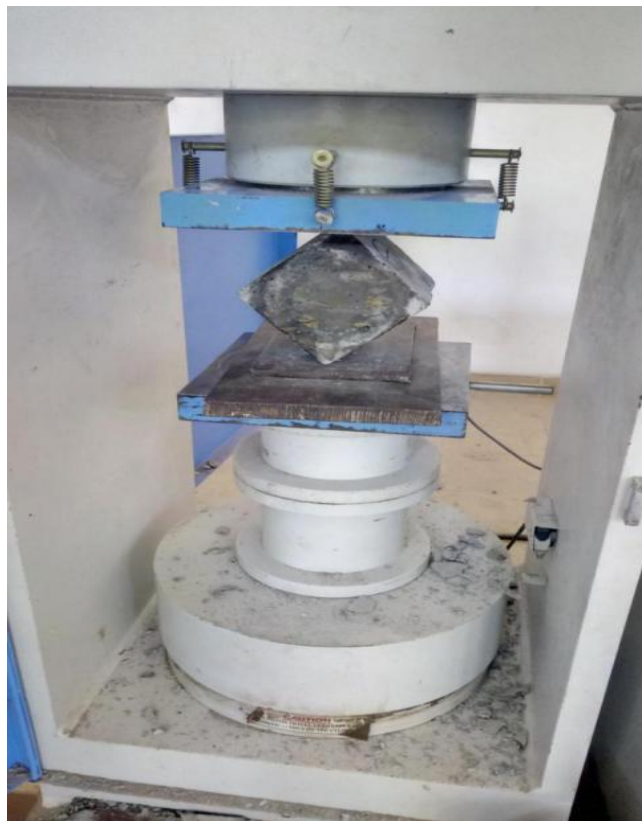
Fig. 3.8 Testing of water permeability sample
