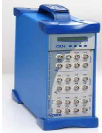
Figure 4.2 Data acquisition system (OR36)
