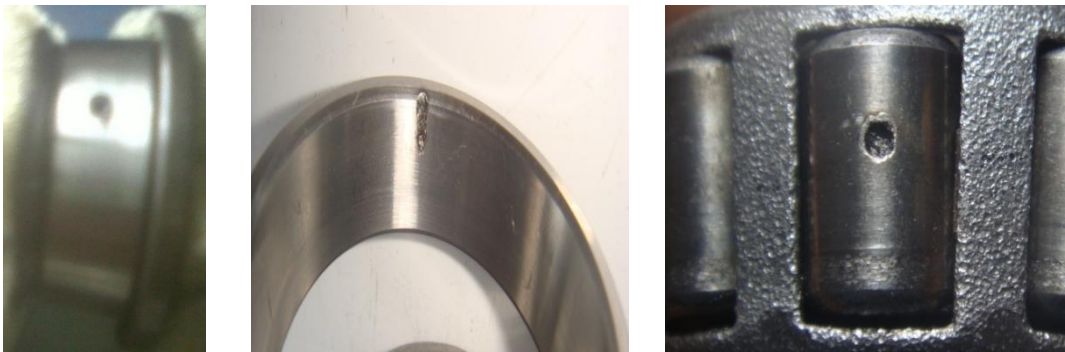
(a) Inner Race with Spall (b) Outer Race with spall (c) Roller with spall
