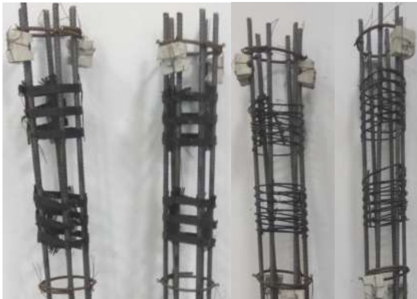
Figure 3.7 Application of geogrids for 450 mm spacing of stirrups
