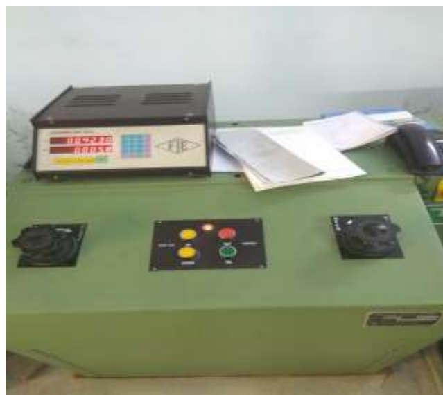
Figure 3.12 Control Equipment for UTM
