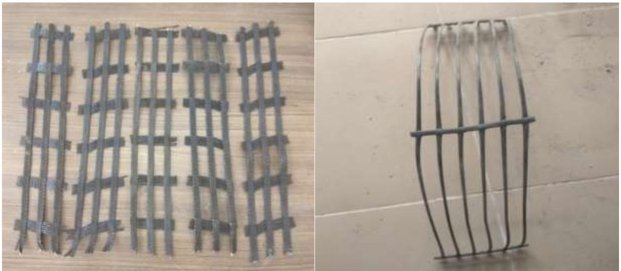
Figure 3.5 Geo-grid strips after being cut for confining purposes
