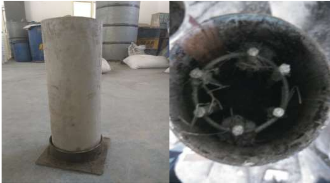
Figure 3.8 Mould used for casting purposes along with top view showing steel reinforcement
