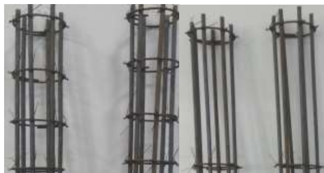
Figure 3.3 Reinforcement cages with spacings 150 mm and 450 mm
