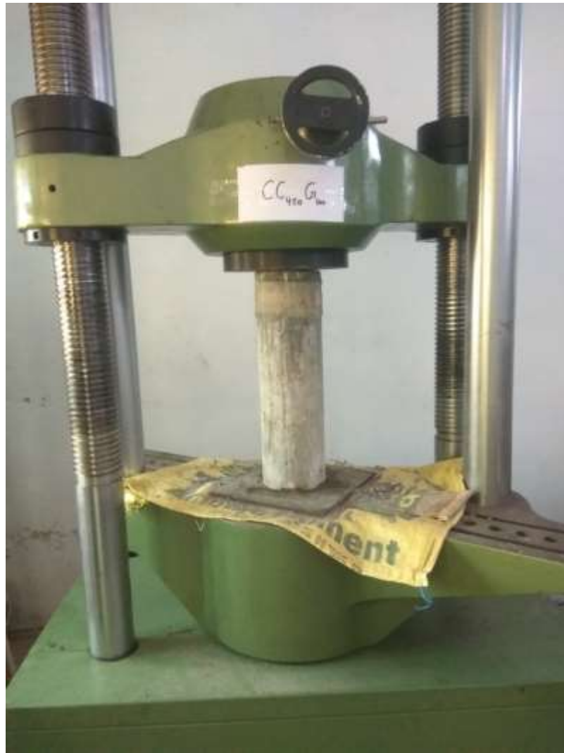
Figure 3.11 Test setup for columns (UTM)
