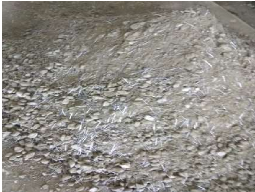
Figure 3.2 Steel fibres dry mixed uniformly
