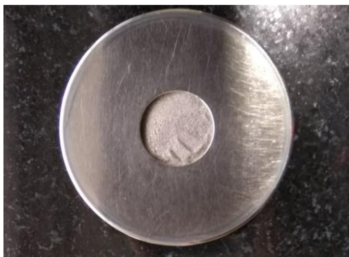
Figure 3.6. Sample holder for XRD.
