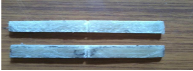
Fig. 33: Specimen breaks under impact load
