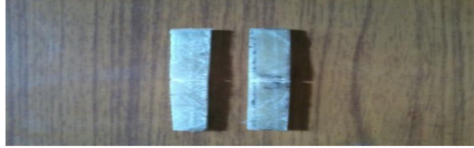
Fig. 31: Specimen breaks under impact load
