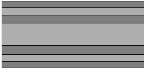
Figure 1.10: Representation of a W1 1-D photonic crystal waveguide structure
