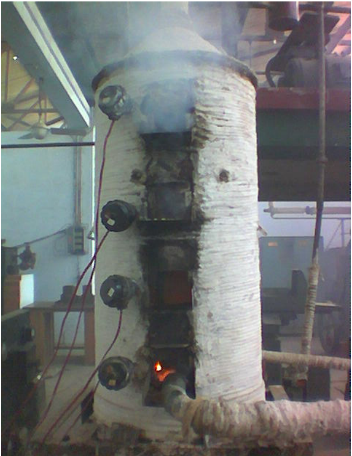
Fig. 5.7-(a )Window 2 being utilized to test the firing order
