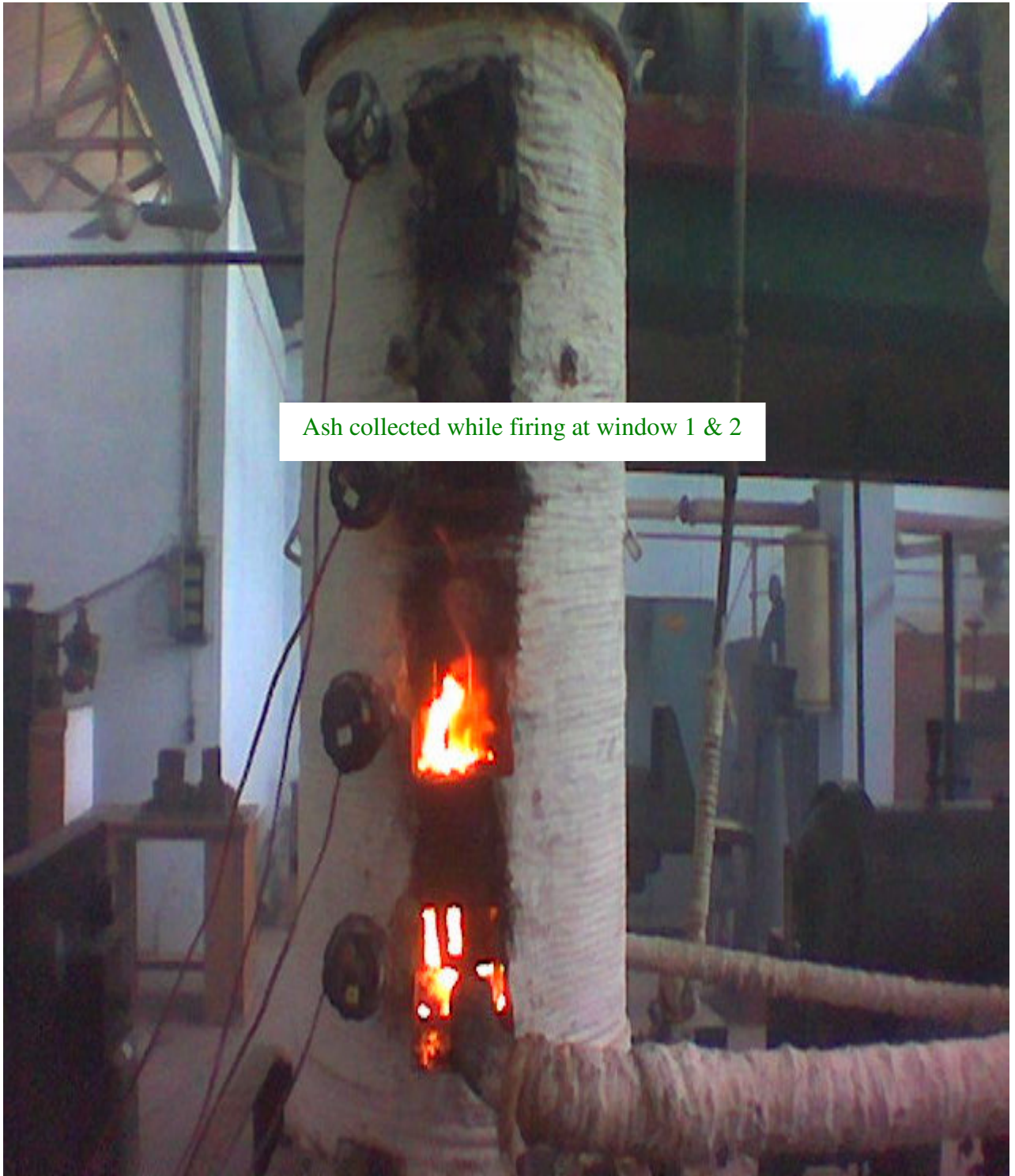
Fig. 5.7-(c) : Window 4 being utilized to test the firing order
