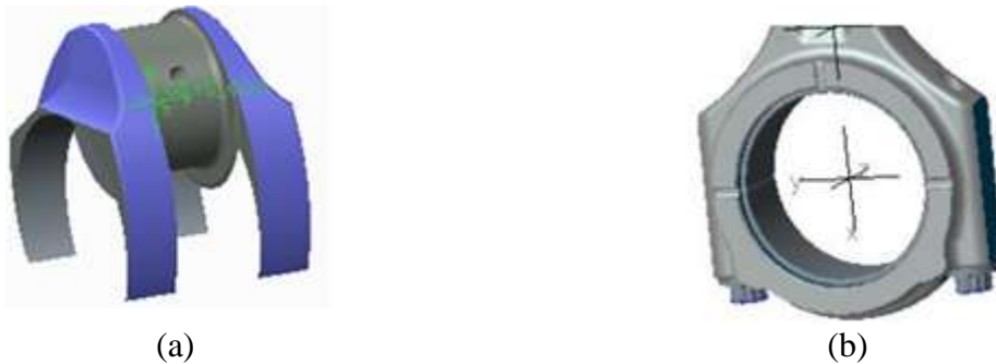
Fig. 3.13 (a) Rotational mass of crank for one throw and (b) Connecting rod big end, obtained from Creo 3.0 software
