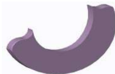
Fig. 3.14 Counterweight profile with 90 kg mm unbalance value, obtained from Creo 3.0 software
