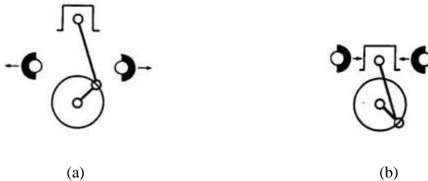
Fig. 4.5 Two balancer shafts cancel out lateral forces
