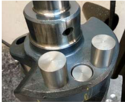
Fig. 1.6 Heavier material is added into the counterweights [6]
