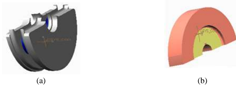
Fig. 3.11 (a) Front balancer mass and (b) Rear balancer mass of balancer shaft, obtained from Creo 3.0 software
