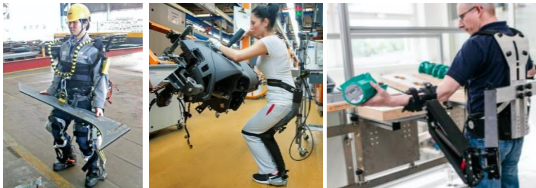
Fig. 2.6: Workers using exoskeletons in various industrial applications [35, 36, 37]
