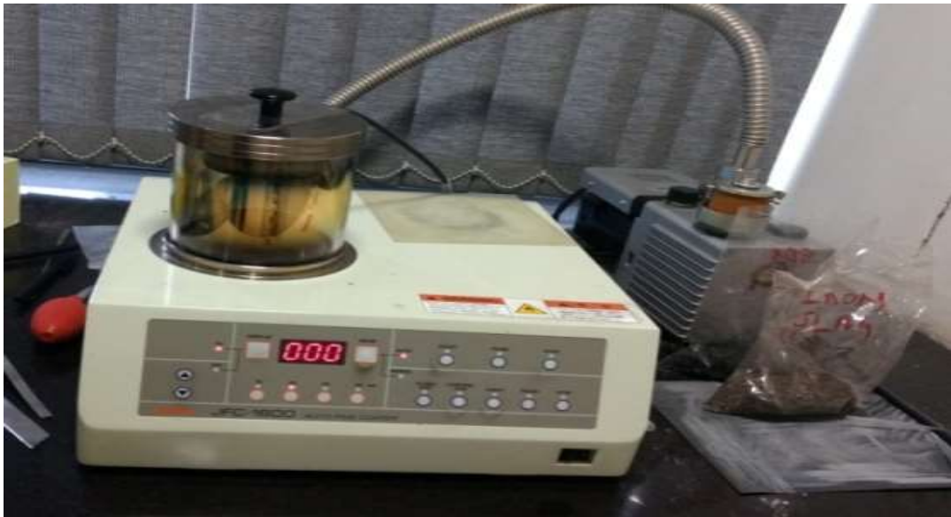
Fig 3.11 Gold plating of sample for SEM
