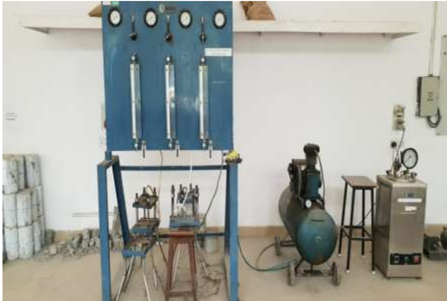
Fig 3.7 Water Permeability apparatus
