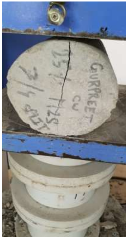
Fig 3.6 Testing of cylinder in CTM for Split tensile strength
