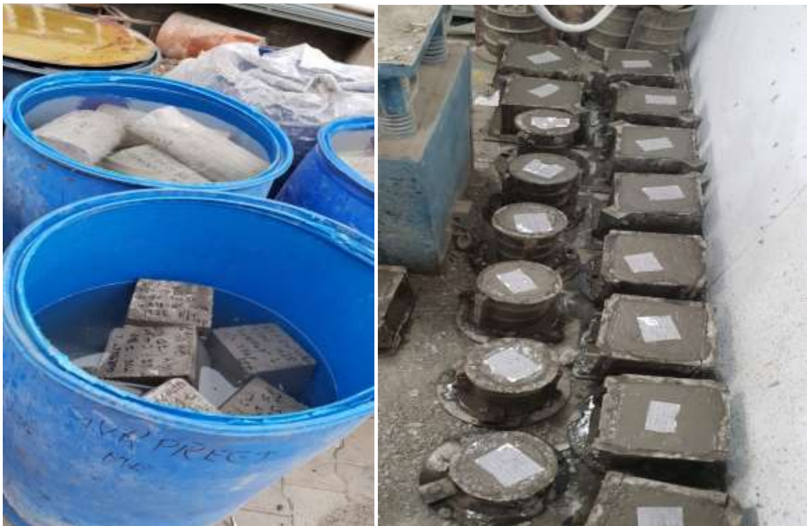
Fig 3.2 Curing and casting of Test specimens
