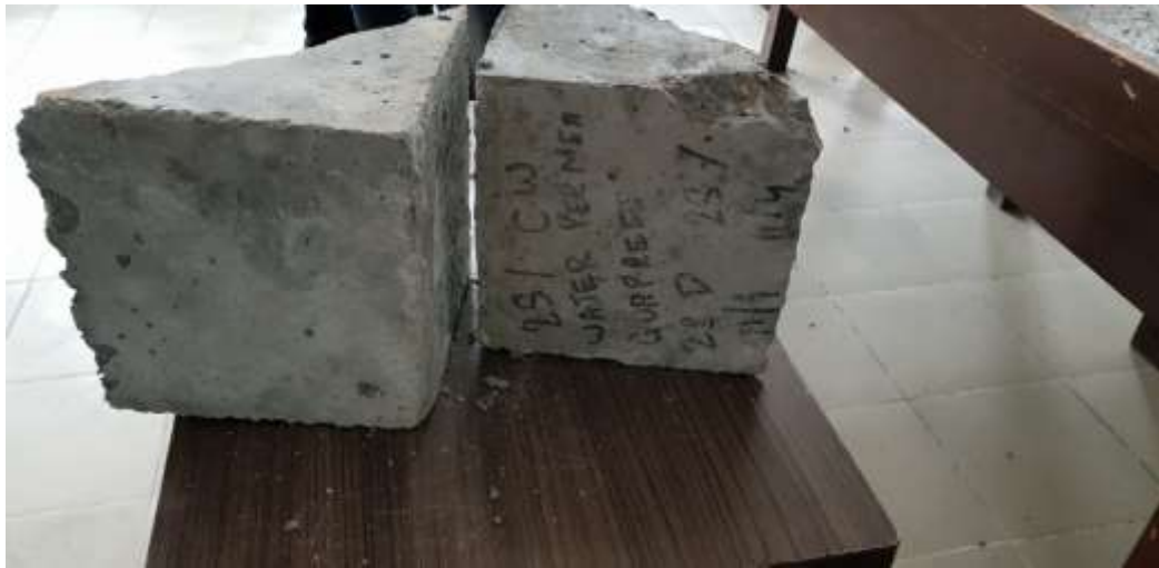
Fig 3.8 Specimen broken into two parts for measuring water penetration depth
