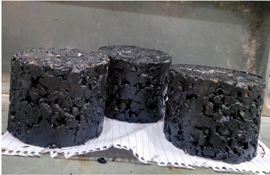
Figure 3.5 Marshall Specimen of SMA mix with Cellulose Fibre
