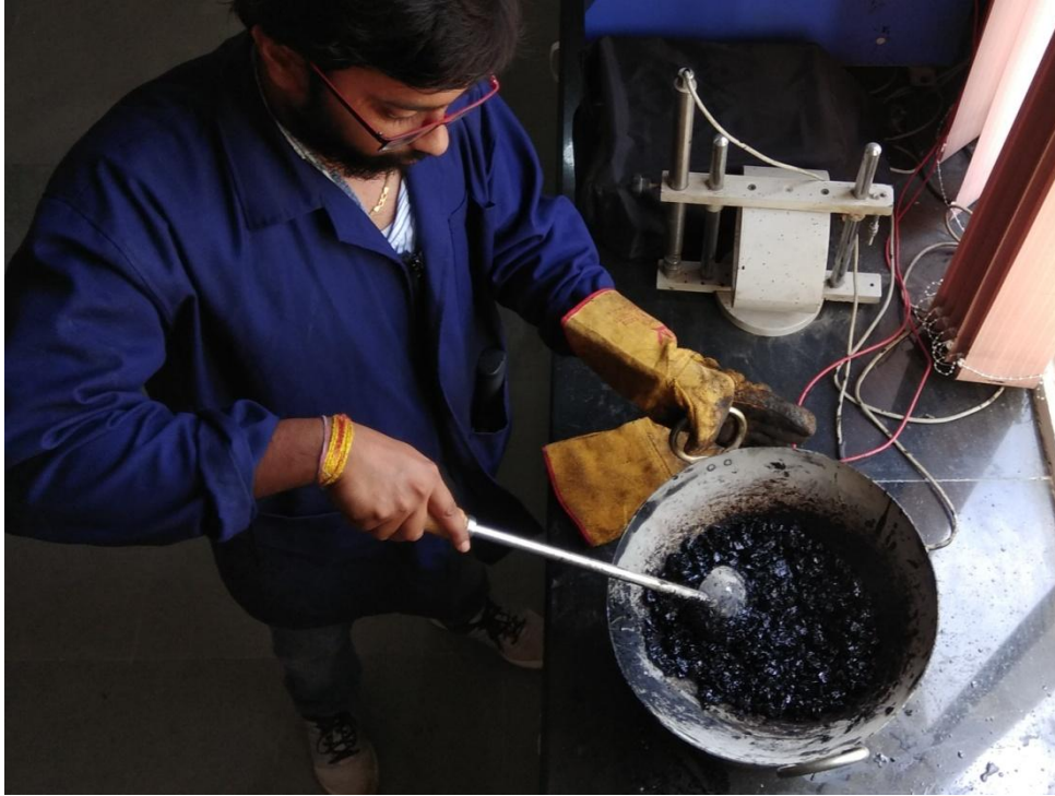
Figure 3.3 Mixing of Aggregates and Binder
