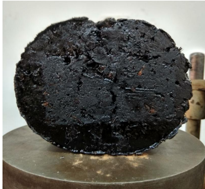
Figure 4.21 Failed Specimen due to ITS Test
