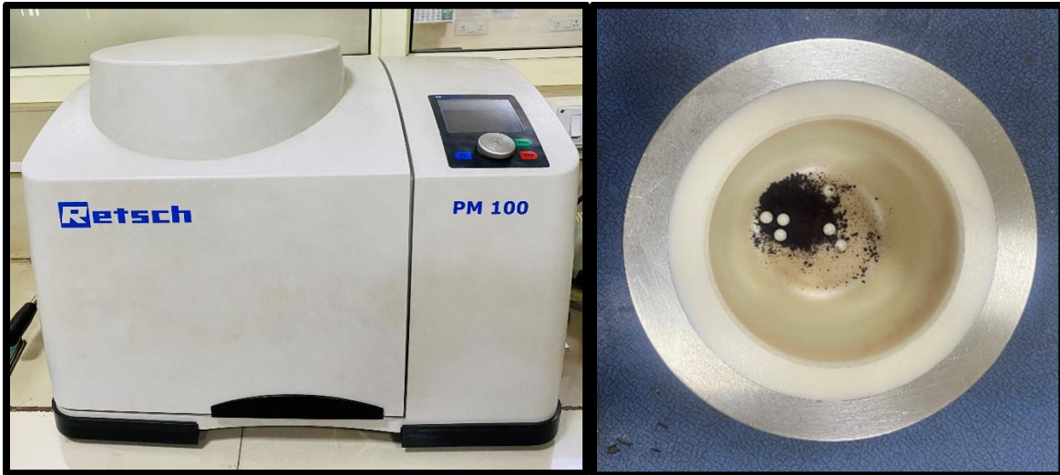
Fig. 3.1 Planetary Ball mill and Zirconia jar with M-Y sample.
