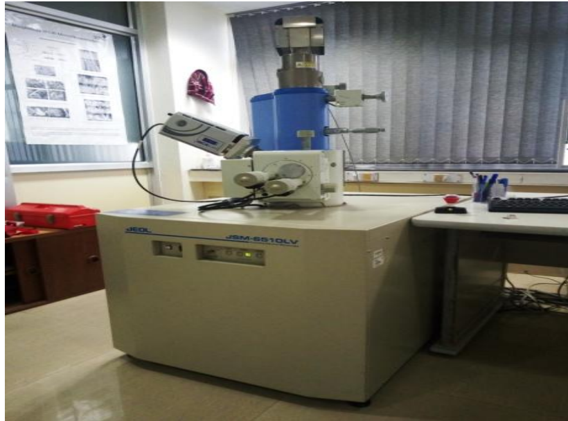
Fig. 3.22: Experimental set up for Scanning Electron Micrograph
