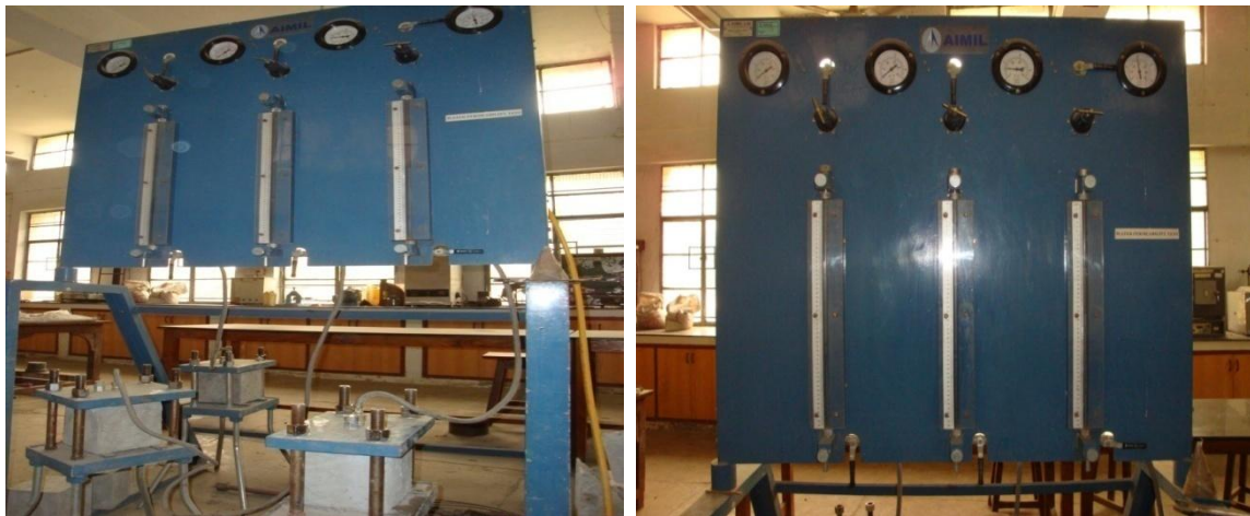
Fig.3.21: Depth of water penetration measurements (WPTM) (from Structure lab TI, Patiala)
