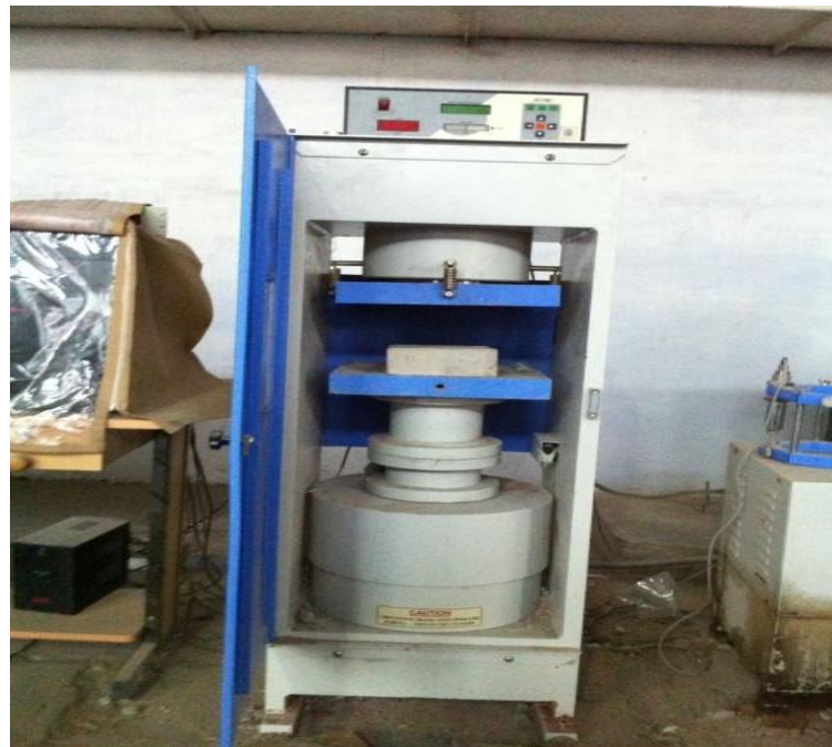
Fig. 3.2: Automatic compression testing machine (courtesy: Structure lab TI, Patiala)
