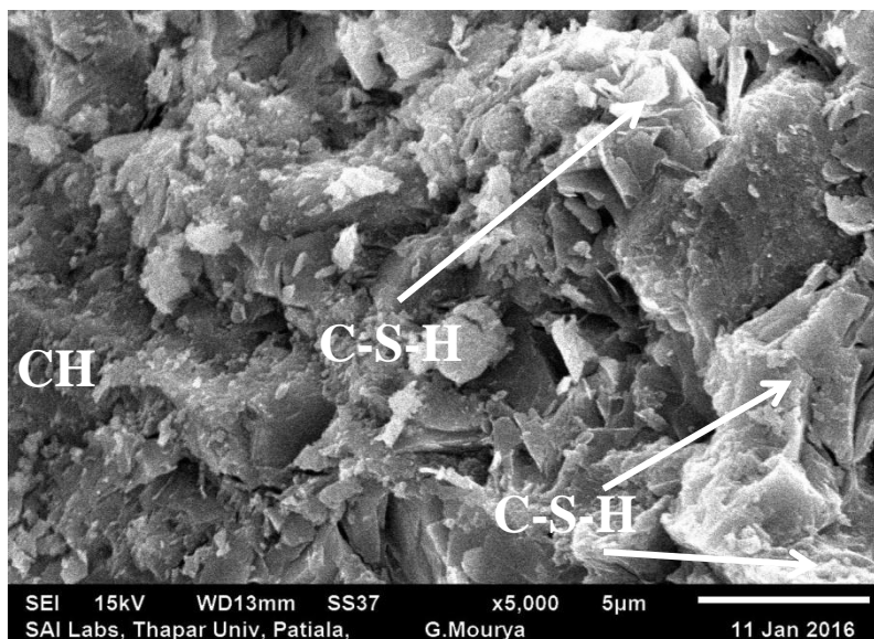
Fig. 5.8: SEM of optimal mix concrete consisting of 10% fly-ash and 30% electric arc furnace slag for w/b=0.48 at 28 days curing age
