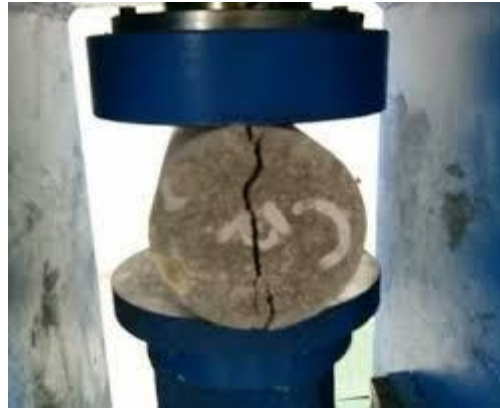
Fig. 3.20: The position of specimen and the type of failure in split tensile test in Automatic compressions testing machine (courtesy: Structure lab TI, Patiala)
