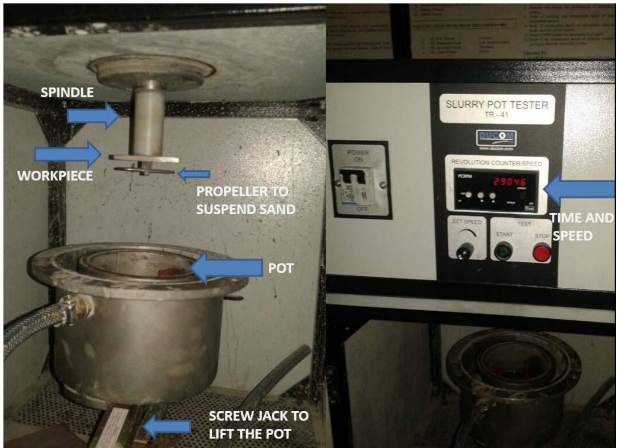
Figure 4.2: Parts of the slurry pot tester
