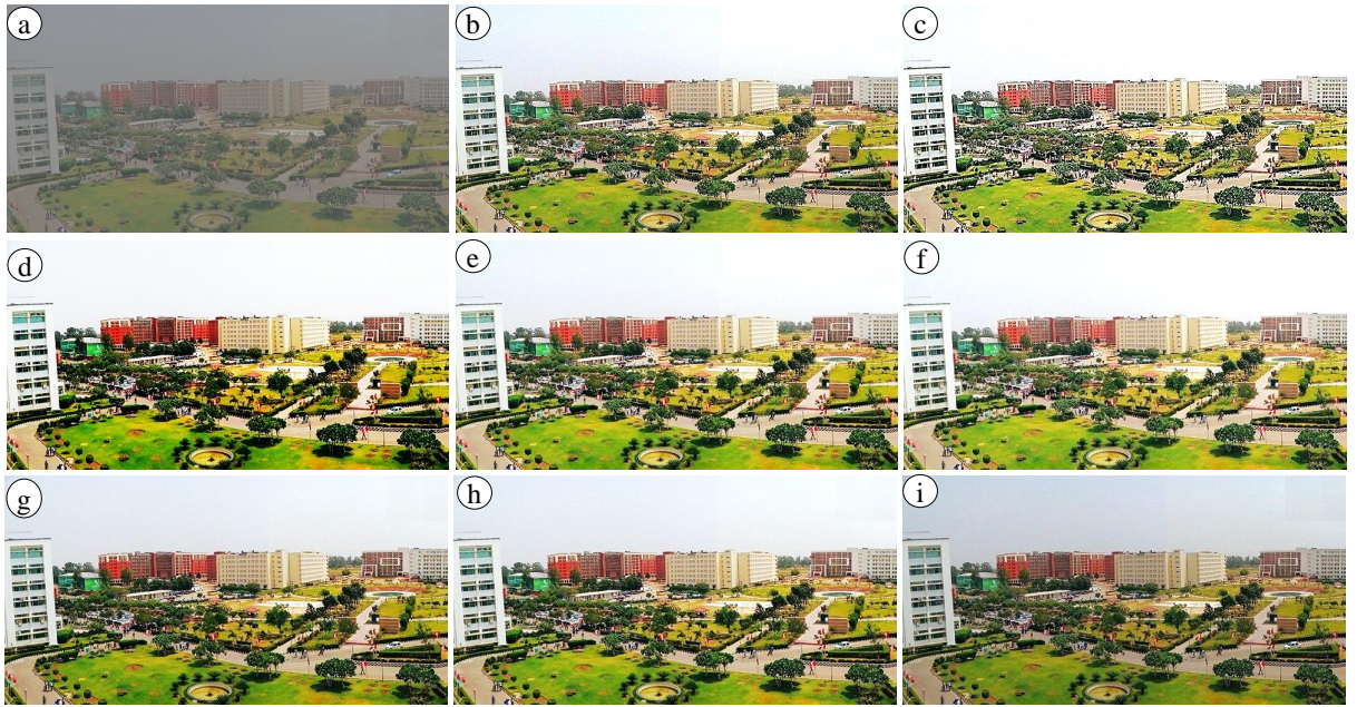
Figure 6.22: Haze removal techniques for tree image (a) Input image (b) DCP, (c) LTQ, (d) MDF, (e) GITF, (f) IVRM, (g) FPDETF, (h) WHDR, and (j) OGPP.
