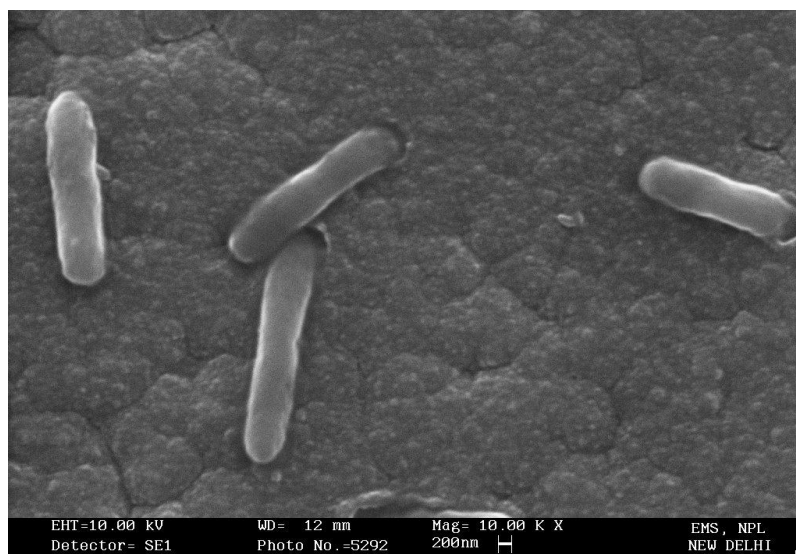
Fig 33 Scanning Electron Micrograph (10 K X) of chrono-potentiometrically entrapped lyophilized biomass of Bacillus sp. MD028 and GLDH on PPy-PVS/ITO electrode.
