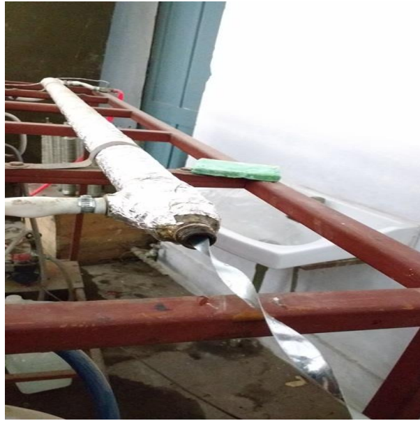
Figure 5.10: Twisted tape being inserted into the inner tube
