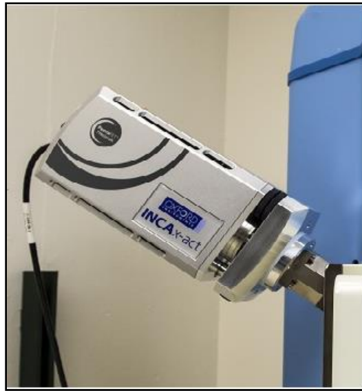
Figure 3.6: EDS attached with SEM
