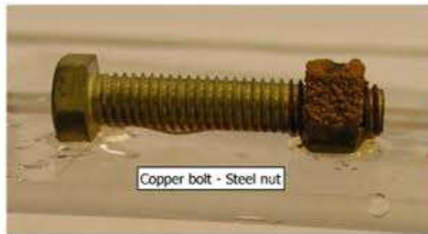
Figure 1.8 Example of Galvanic corrosion ( http://www.tecnoconverting.com )
