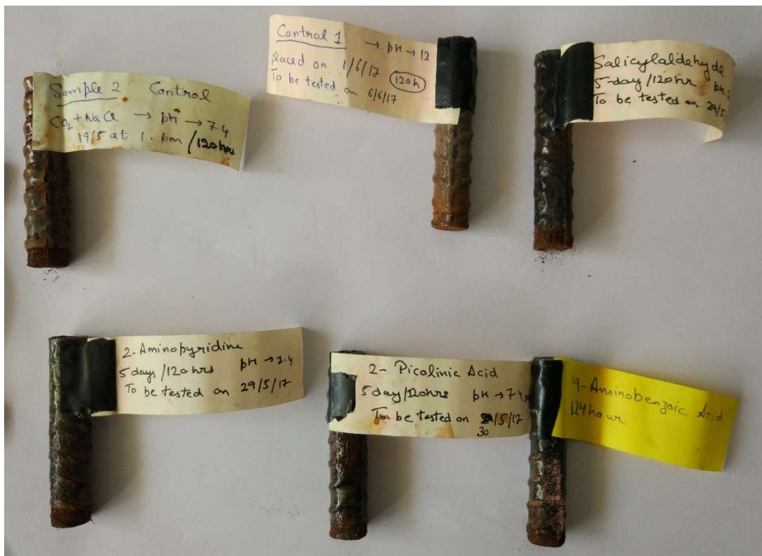
Figure 5.7 Steel specimens after measuring Half-cell Potential and Linear Polarization Resistance, immersed partially in different solutions after 120 hours
