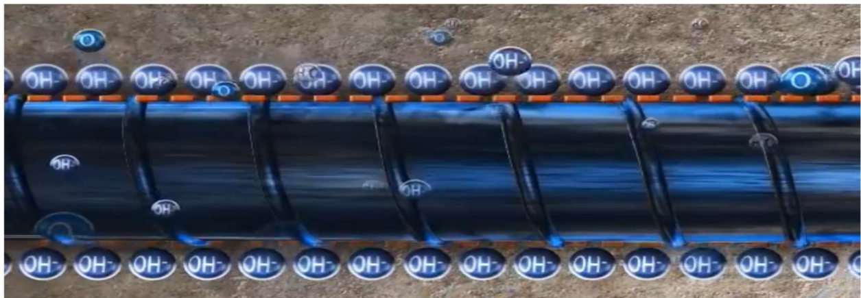
Figure 1.2 Layer of \text{Fe(OH)}_3 film formed around Steel bar ( http://chemblinks.blogspot.in )
