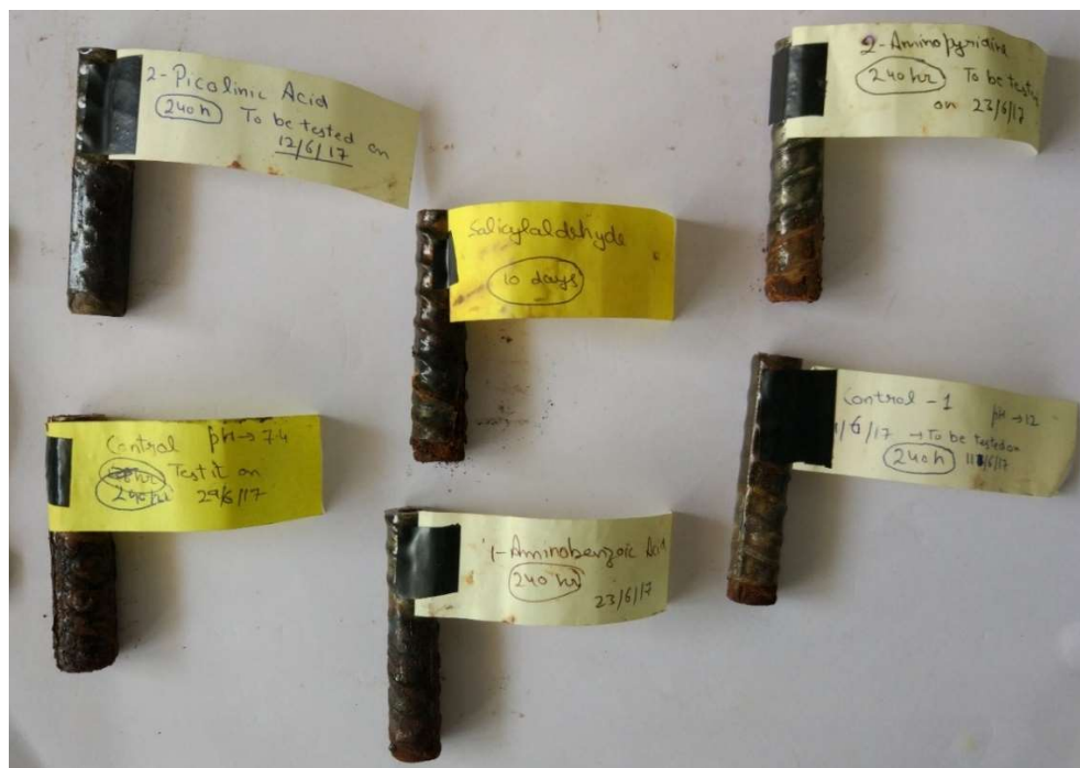
Figure 5.9 Steel specimens after measuring Half-cell Potential and Linear Polarization Resistance, immersed in different solutions after 240 hours
