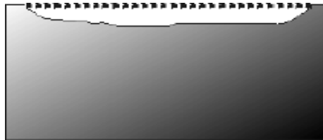
Fig 3.7 Uniform Corrosion (www.corrosion-doctors.or)
