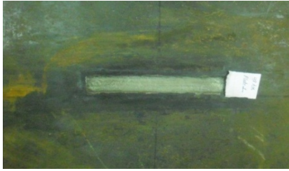
(a) After 2 days corrosion
