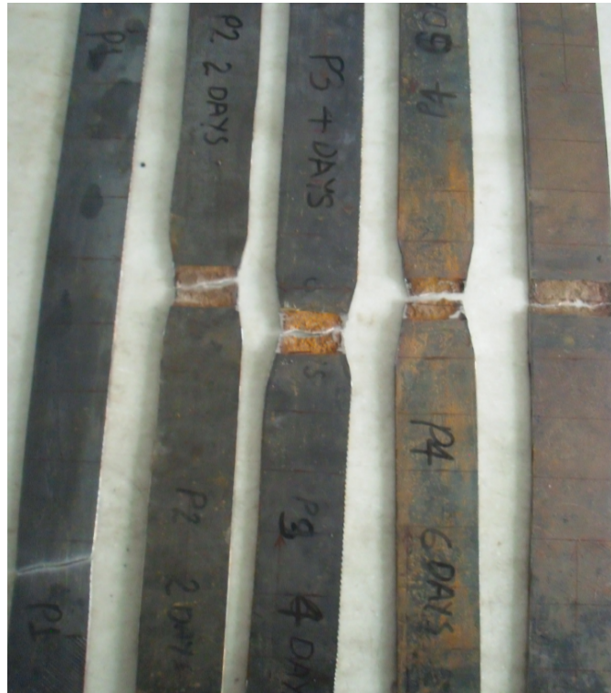
Figure 4.23 Failed tensile test specimens at different ages of corrosion
