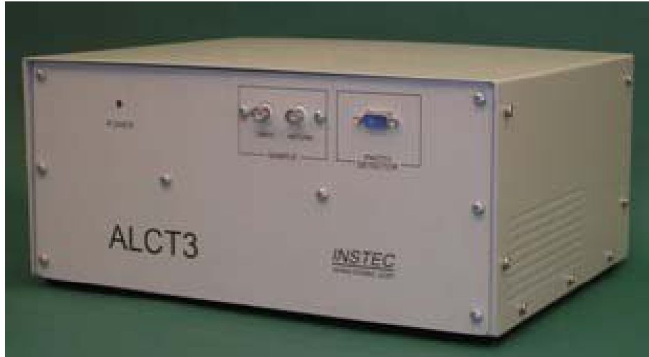
Fig2.10: ALCT meter used to study the value of P_s and viscosity.
