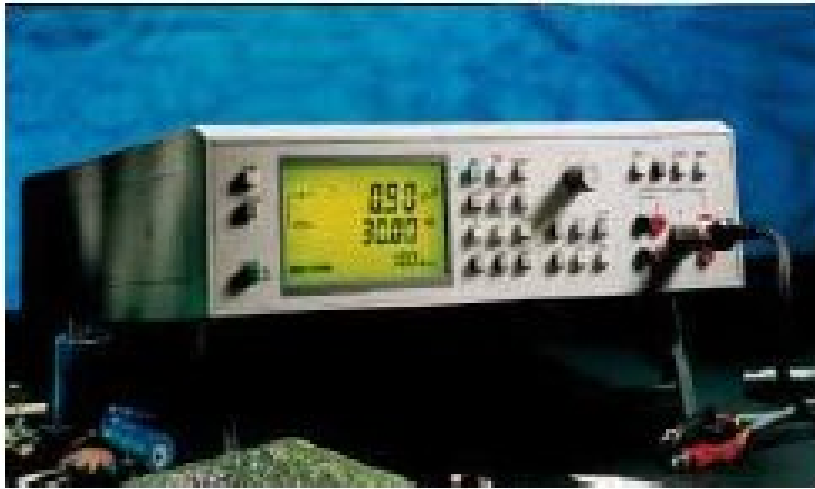
Fig. 2.9: Programmable automatic RCL meter [FLUKE PM6306] used for dielectric studies.
