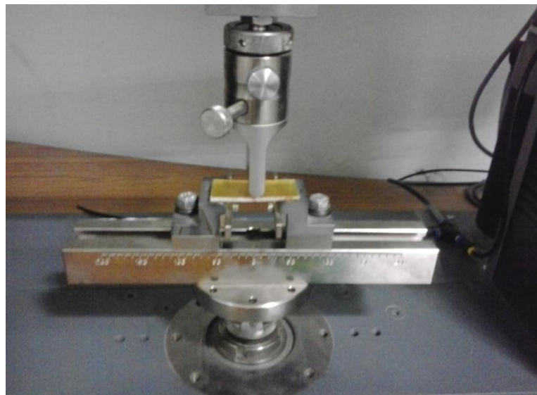
Fig. 3.5 Specimen positioning in three point bend test on UTM
